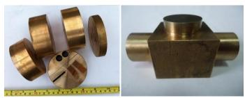
Figure 1. W-Cu materials prepared by combustion synthesis and centrifugal infiltration
