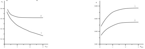
Fig. 1 Critical conditions for the ignition. Fig. 2 The burning rate u vs. the gravity  $A_{grav}$ . External heat exchange  $B_0=0.001$  (1);  $B_0=0.002$  (2) Q=0.2 (curve 1), Q=0.1 (curve 2)
