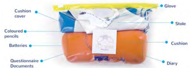
Figure 3: The Felt Sense Kit. The main devices were composed of a glove with haptic stimulation to anchor the felt sense, a cushion with a pulse sensor that generates vibration as it were an externalisation of the user's heartbeat and a stole painted with thermochromic ink that disappears in contact with human touch.
