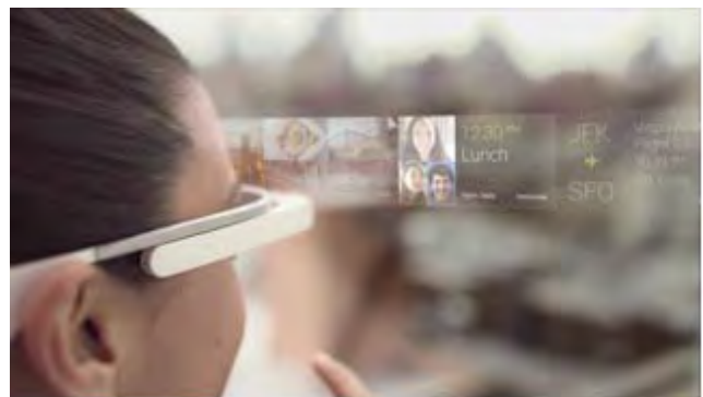
Figure 2. Google Glass, simulated view of data "timeline" overlaid on normal view. Google photo.
