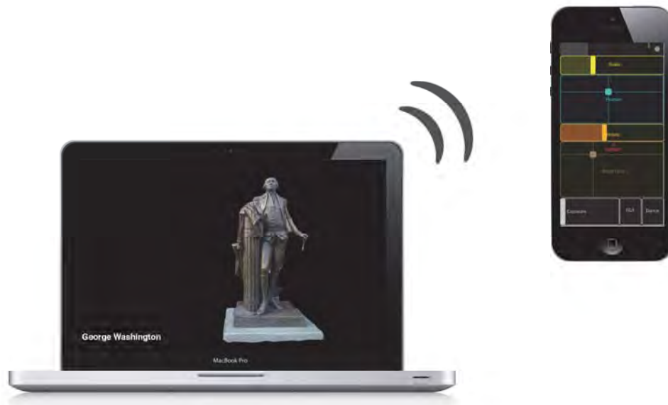
Figure 6. Statuevision Software: Models are animated on the computer screen in real time, controlled by the custom mobile application.
