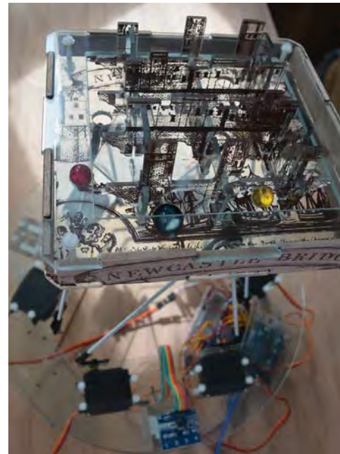
Figure 1. Gesture Puzzle 1: Newcastle Bridge . Glass, enamels, wood, capacitive touchpad, Arduino microcontroller, servomotors. Hursty, Bradbury. 2015.
