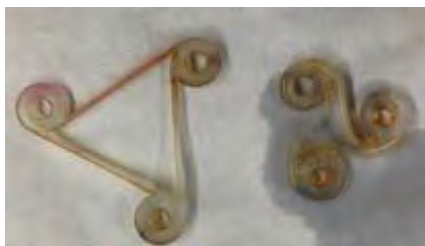
Figure 2: Contraction of Chiral Structure: Expanded ( left ) and Compressed States ( right )
