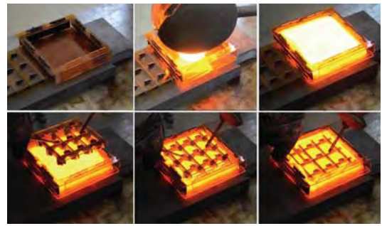
Figure 6. Montage of pressing molten glass into a sheet glass Puzzle Box . Hursty, 2014.
