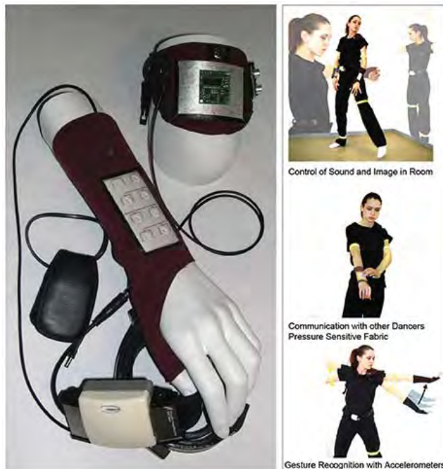
Fig.6 Stage Three of «eskin»: Mobile wearable armband interface, embroidered circuit, sensors and shoulder pad hooked up to the QBiQ computer from the Wearable Computer Laboratory. Swiss Federal Institute of Technology. Design Jill Scott (2008)
