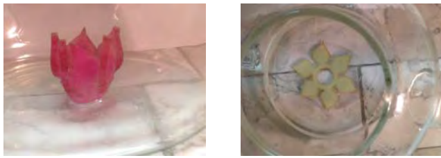
Figure 5: Left : SMP Flower Before Exposed to Hot Water, Right : SMP Flower After Exposed to Hot Water
