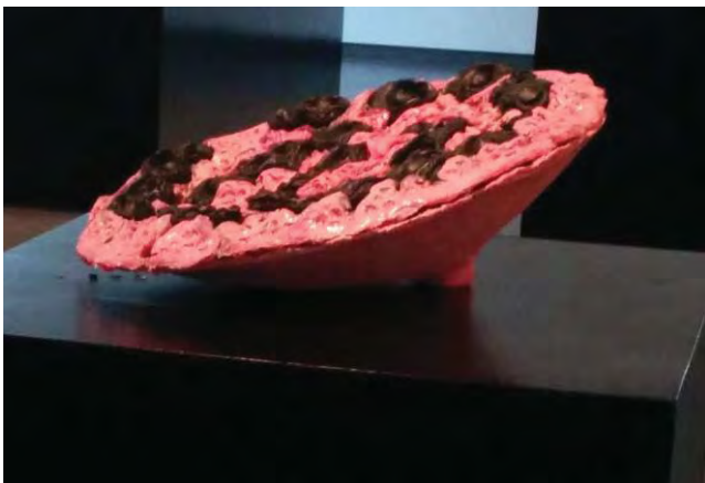
Figure 2. The Silicone Valley . The black hard plastic elements protruding from the breast tissue concentrate the vibration feedback and host the conductive copper wire of capacitive sensors.
