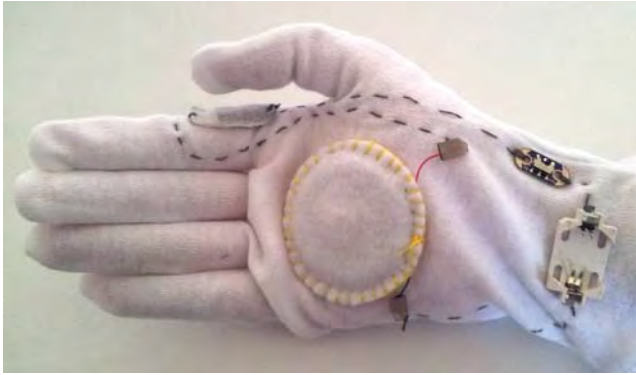
Figure 2: After the pilot testing session, the LEDs were removed and the device simplified to haptic stimulation. The pushbutton to control the stimulus was relocated between the thumb and the low portion of the index finger.
