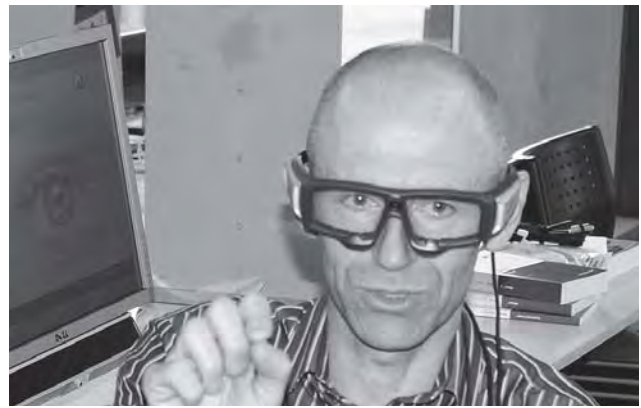
Figure 1. Tracksys ETG 60Hz binocular tracking glasses.
