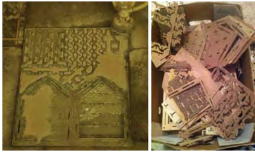
Figure 7, left . Waterjet cutting glass with disposable wooden backing board underneath. Hursty, 2014
