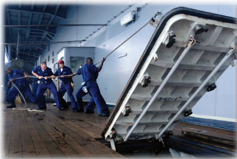
PACIFIC OCEAN (Aug. 15, 2008) Sailors assigned to the engineering repair division aboard the amphibious command ship USS Blue Ridge (LCC 19) raise an external hatch to perform maintenance on the watertight gasket and moving parts. Blue Ridge is the flagship for Commander, U.S. 7th Fleet. (U.S. Navy photo by Mass Communication Specialist 2nd Class Peter D. Lawlor/Released)
