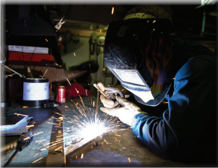
PACIFIC OCEAN (Jan. 31, 2013) Hull Maintenance Technician 3rd Class Jesse Belfi strikes a welding rod to mend the hinge of a quick-acting watertight door handle aboard the amphibious assault ship USS Bonhomme Richard (LHD 6). The Bonhomme Richard Amphibious Ready Group, deployed in the U. S. 7th Fleet area of responsibility, will take part in amphibious integration training (AIT), certification exercise (CERTEX), and participate in the annual multi-national combined joint training exercise Cobra Gold. (U. S. Navy photo by Mass Communication Specialist 3rd Class Amanda S. Kitchner/Released)
