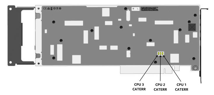
Figure 5. Light Guided Diagnostics - Processor CATERR LEDs
