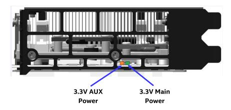
Figure 4. Light Guided Diagnostics - Power State LEDs
