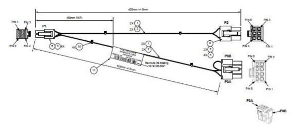
Figure 8. Auxiliary 12V Power Cable (iPC AXXGPGPUCABLE)
