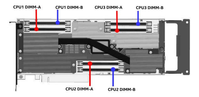
Figure 3. VCA Card DIMM Slots
