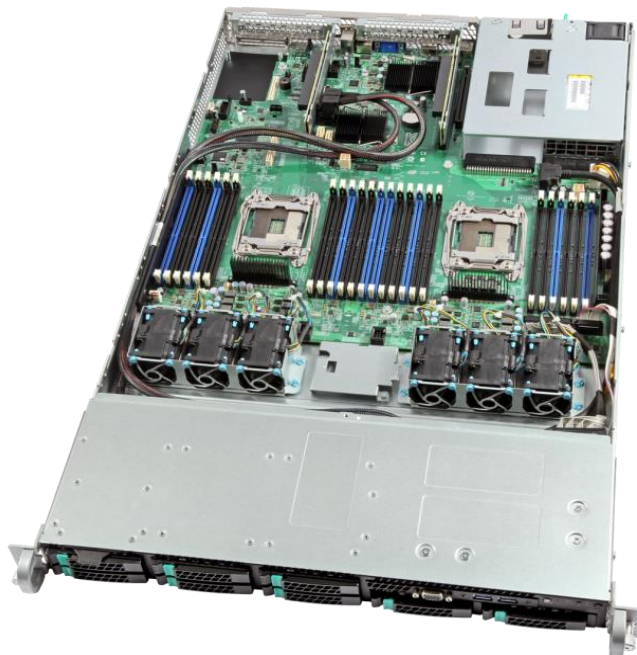
Figure 5. Intel® Server System R1000WT – L6 Integrated 1U System *R1208WTxxx shown
