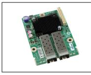
AXX10GBNIAIOM 917905 735858241090 5032037035842 Dual SFP+ port 10GbE IO module based on Intel® 82599 10 Gigabit Ethernet Controller Supports direct connect or transceiver.
