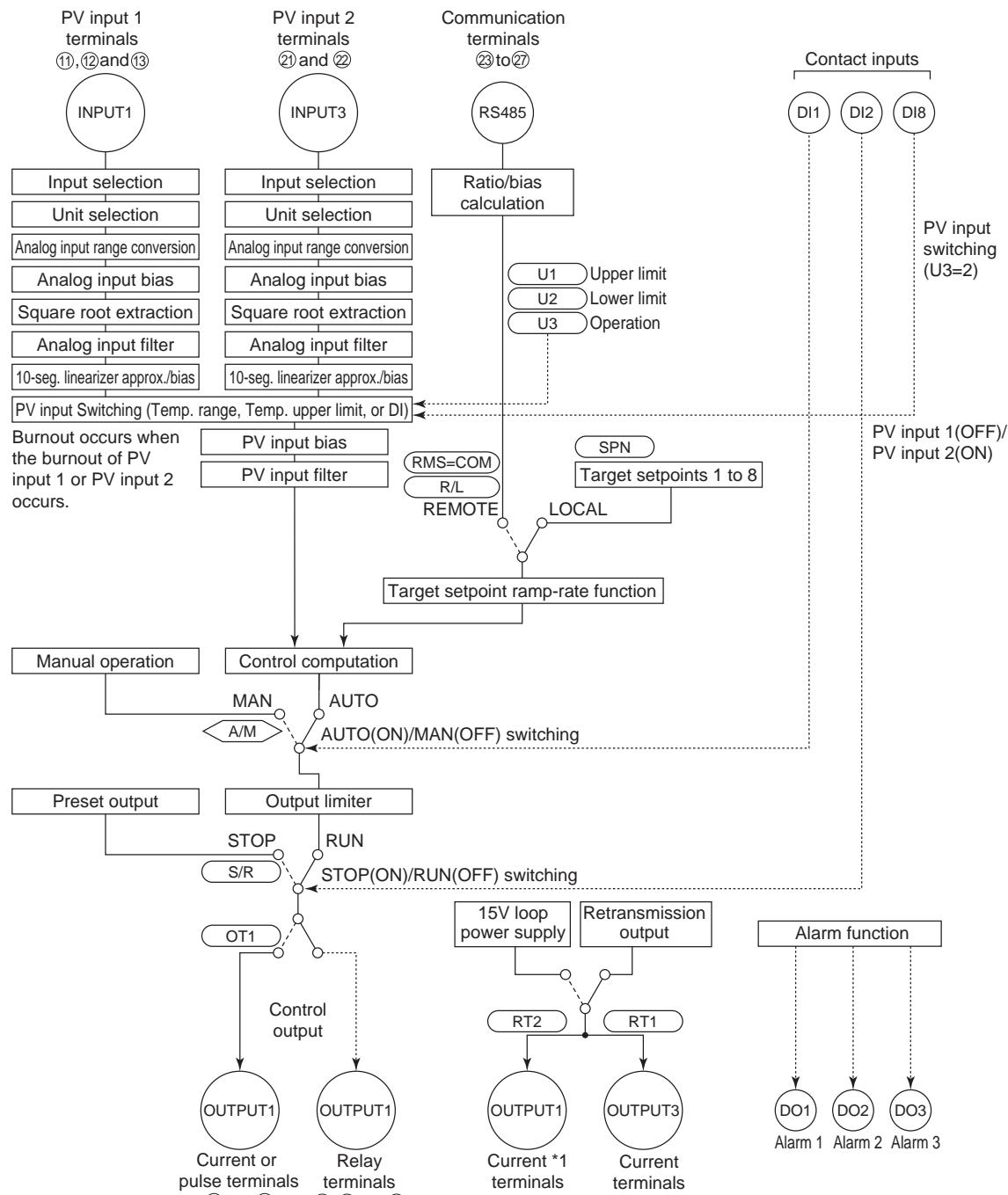
\*1 Unavailable when control output is current or pulse.
