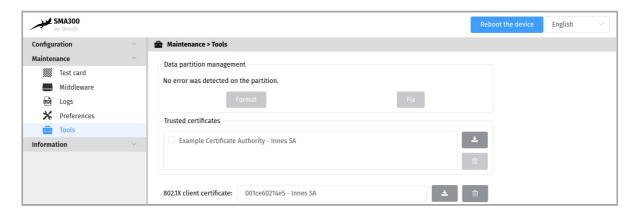
■ The format and fix buttons are only active if the Gekkota OS middleware has actually detected write or read errors on the partition.
