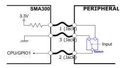
Two wires configuration for GPIO1:
