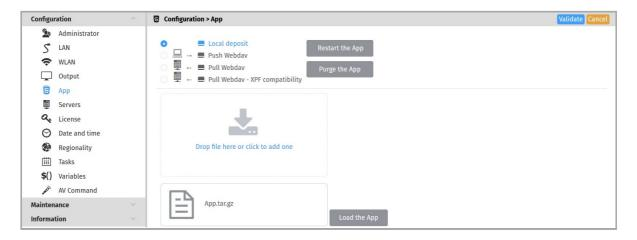
Then click on the Load App button. When the file disappears from the interface, the App is loaded and starts automatically.
