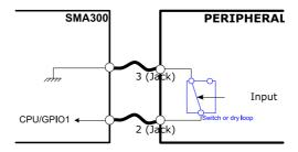
Output configuration for GPIO1:
