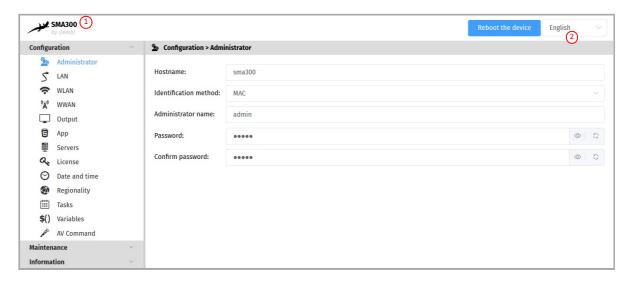
After you have changed and saved all your settings in the different panes, be sure to perform a device restart by clicking on the Reboot the device (2) button so that your changes are fully reflected.
