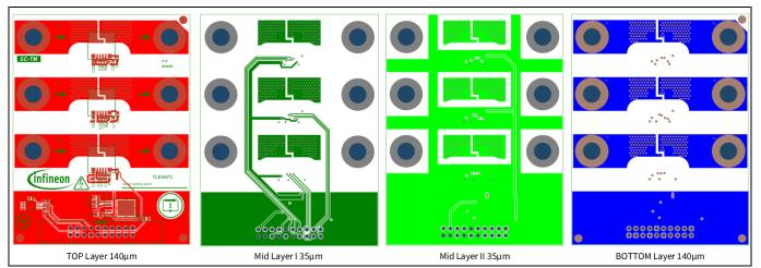
Figure 3 Board layout of 4-layer reference board
