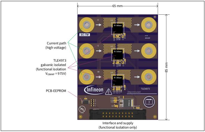
Figure 1 TLE4973 EVAL 120A, three phase measurement board
