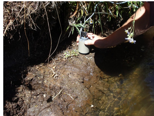
Cohesive Strength Meter for in situ measure of critical shear stress.
