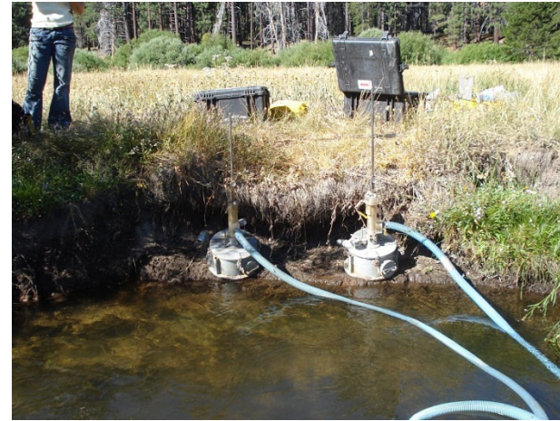
Jet Test for in situ measure of erosion-rate coefficient and critical shear stress.
