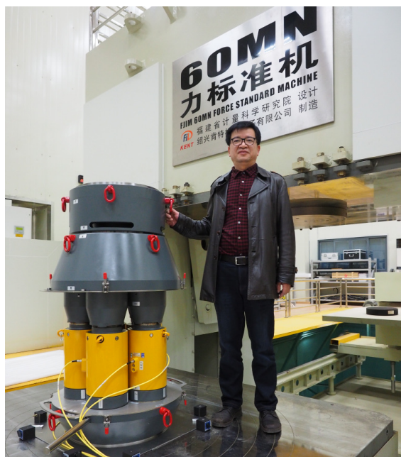
Figure 6: 50 MN BU system and Prof. Yao in front of the 60 MN FSM showing the compact design of the 50 MN BU system.
