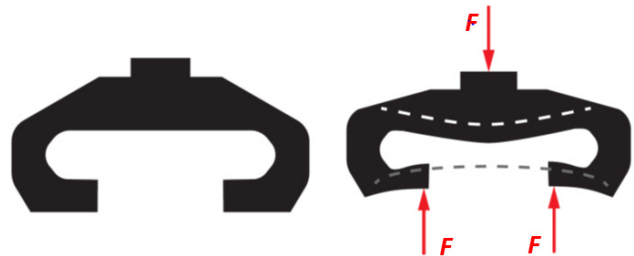
Figure 1: So-called “bending-neutral plate” used to disable cross forces by reducing sideways movements or any tilt angle at the force introduction point under load.
