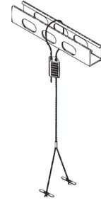
HB-XX-18Y-PAD Y-Toggle Cable System (xx = in)
