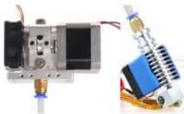
Fig. 17. Example of Bowden extruder, [17]
