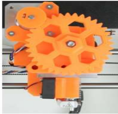
Fig. 16. Example of extruder with gears, [17]
