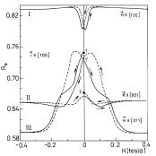
Fig. 1. The effect of magnetic field of different direction on  $U_3As_4$  resistivity along [100]
