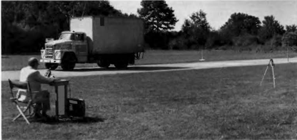
Figure 1-5. Use of Preamplifier Cables in a field application for sound-level measurements.
