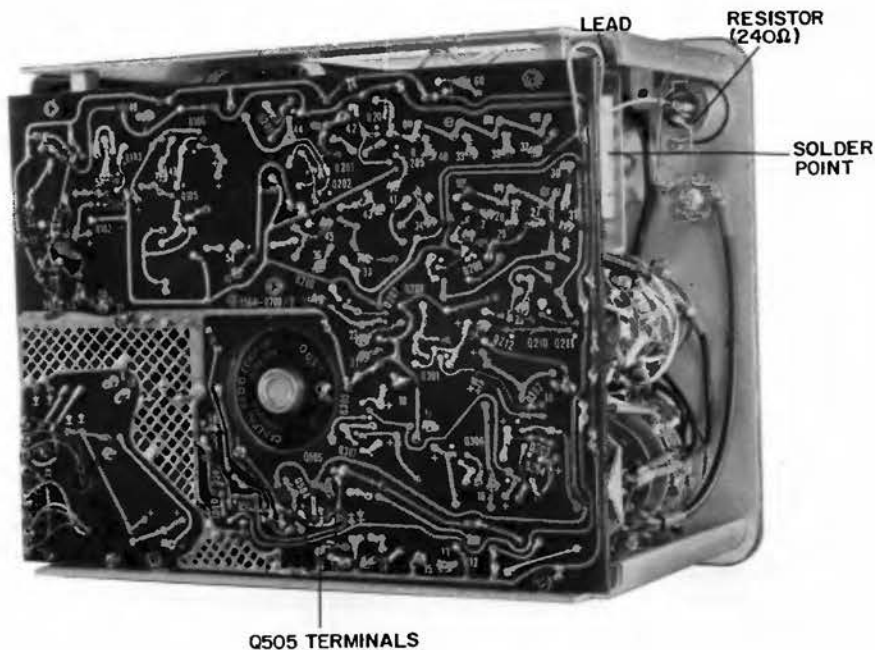
Figure 7-2. Modification of Type 1564-A Sound and Vibration Analyzer for use with the preamplifier.
