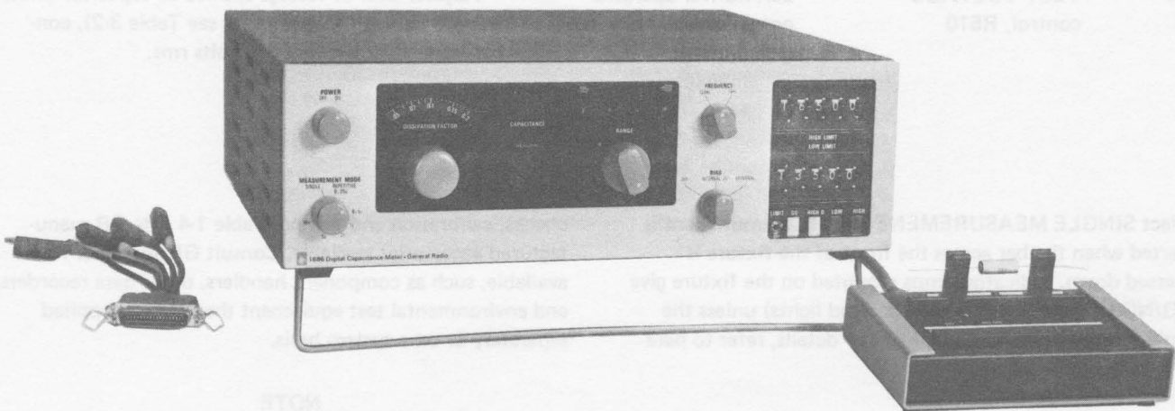
Figure 1-3. Test fixture in use, with adaptors for axial-lead capacitors. The elementary test cable is shown at the left.
