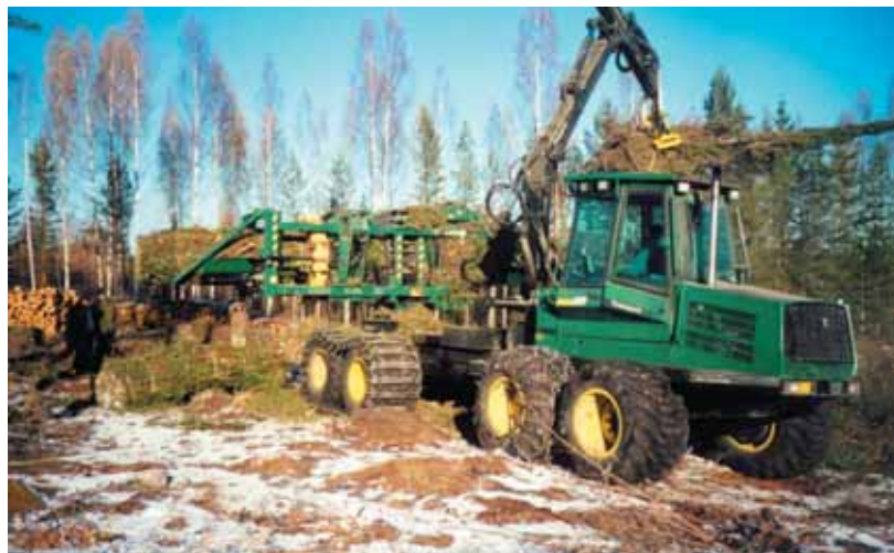
In Finland, the goal is to double the use of renewable energy sources by 2025 and thus contribute over one-third of total energy consumption. This increase will come almost entirely from bioenergy with forest residues being a significant component. The image above shows the Timberjack Slash Bundler manufacturing 'compacted residue logs' after final harvest. (Courtesy Dr Arto Timperi, Timberjack and J Tustin)
