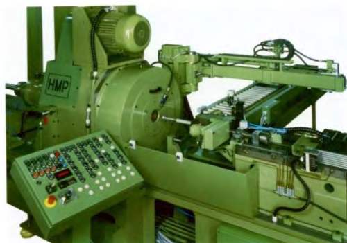
Fig. 6 Rotary forging machine for forming of metallic materials with reduced formability
