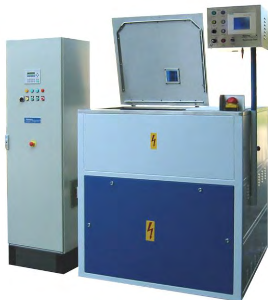
Fig. 3 Induction centrifugal casting unit (firm Linn, Germany) for casting of nickel and titanium alloys, super-alloys etc. (max. casting weight of Ti: 2 kg)
