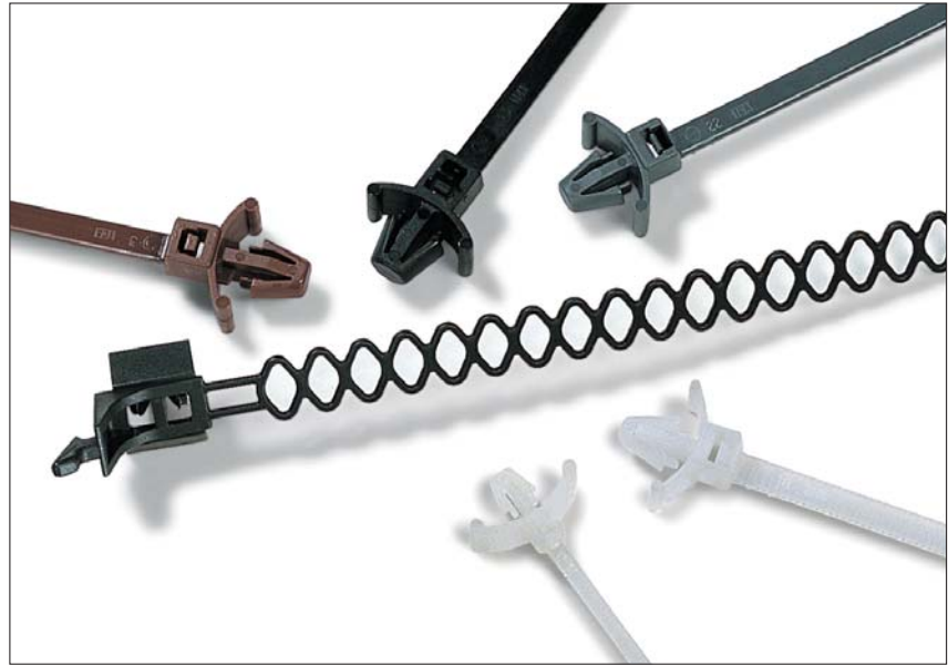
A wide range of arrowhead fixing ties which are suitable for panel thicknesses of 0.5mm to 4.5mm and hole diameters of 4.4mm to 8.0mm.
