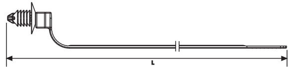
Special design without a gap between head and bundle; FT220DP7
