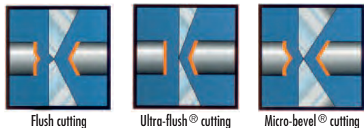
Flush cutting Ultra-flush® cutting Micro-bevel® cutting
