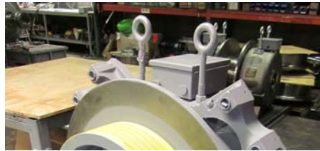
Figure 10: 2 lifting eye bolts installed (example)
