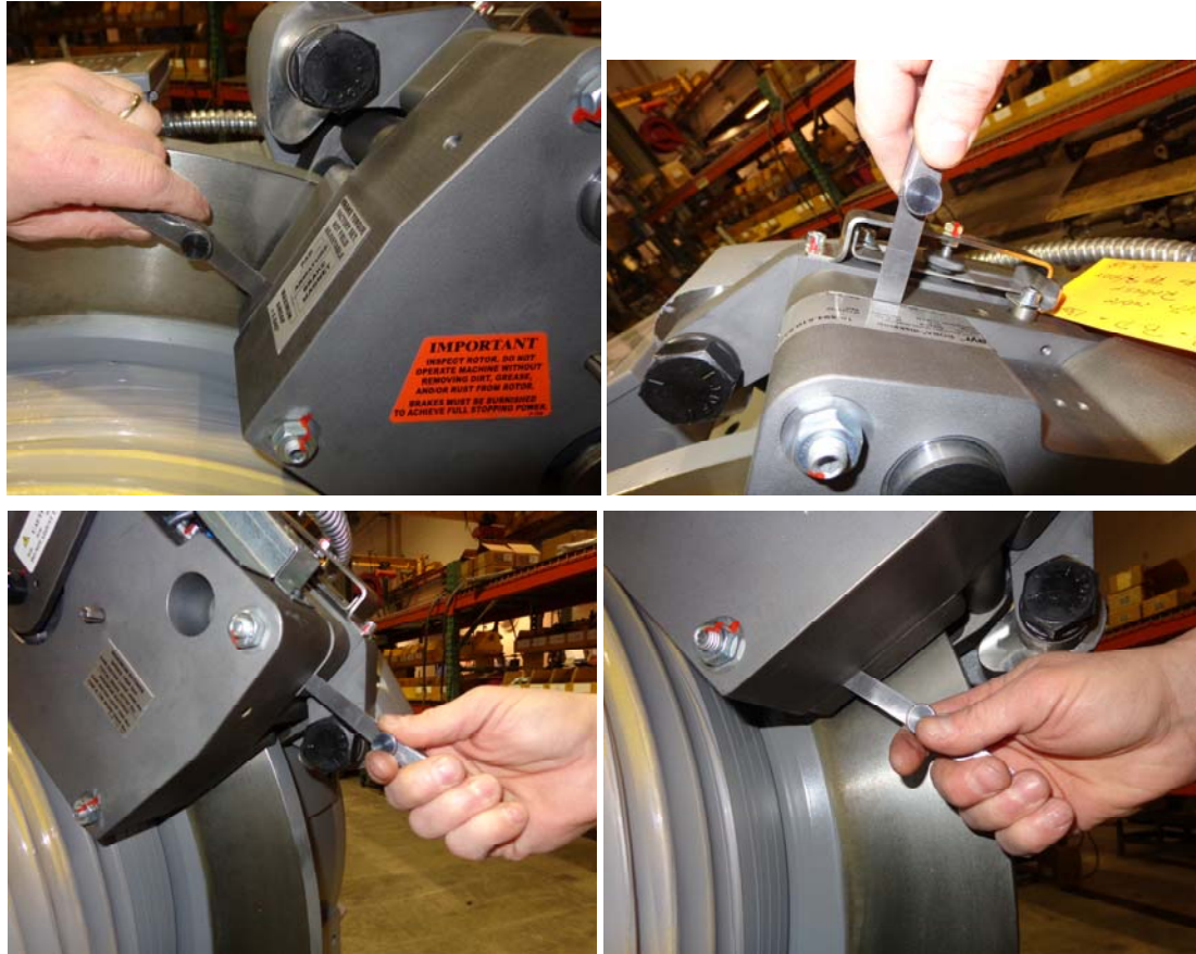
Figure 26: Air Gap readings 4 places around brake.
