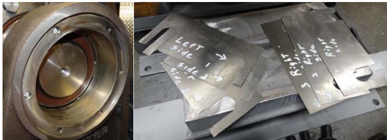
Figure 8: Base Clear of Bearing, and all Shims Marked
