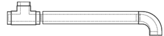
D. Flex carrier elbow and pipe toward tee and weld to carrier tee pipe
