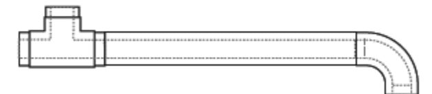
E. Weld containment pipe to containment tee
