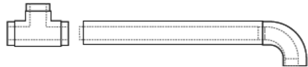
C. Weld containment elbow to containment pipe
