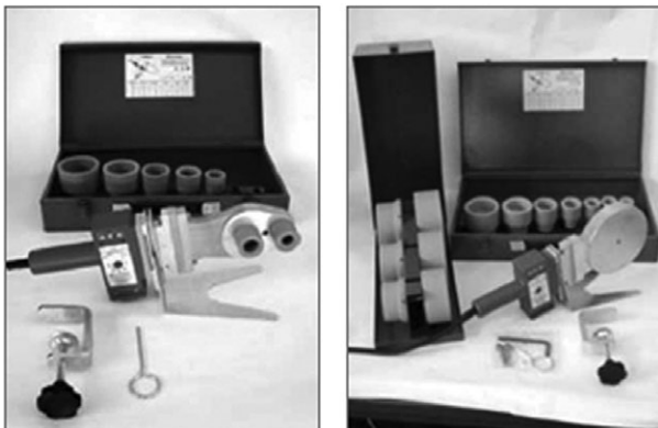
Figure 15 Hand-held socket fusion for ½"-2" show left, 1/2"-4" on right
