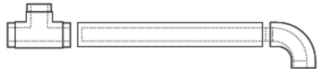
B. Pull carrier elbow out of containment elbow and weld to carrier pipe
