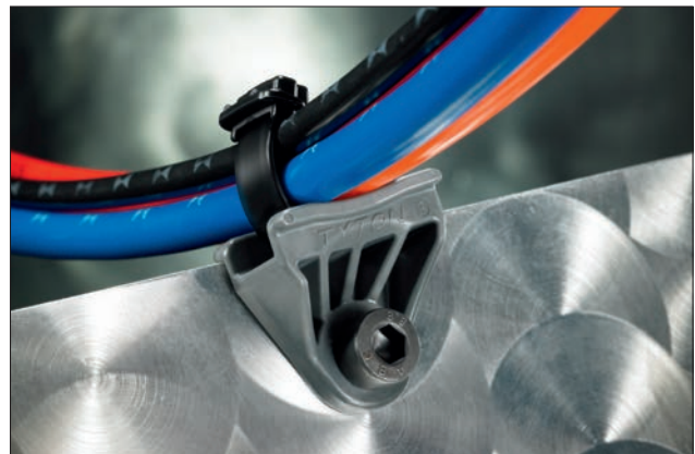
Axial oval mounts stand off bundles from frame rails and cross members to prevent them from rubbing and chafing.
