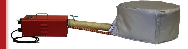
This Portable Hot Air Composite Curing System fills an important gap in composite repair techniques by applying heat to difficult shapes or hard to reach areas. Primary applications are composite repairs, secondary bonding, and modifications to composite structures. Powered and controlled by a Hot Bonder, it provides even heating of contoured surfaces and can be effectively used in place of standard silicone rubber heat blankets.
