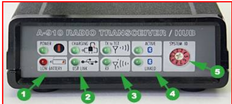
Figure 32 – The A-910 Radio Transceiver/Hub FRONT PANEL
