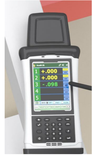
Figure 21 -- R-1356-2.4ZB PDA Readout showing data values for Targets #1, 2 and 3
