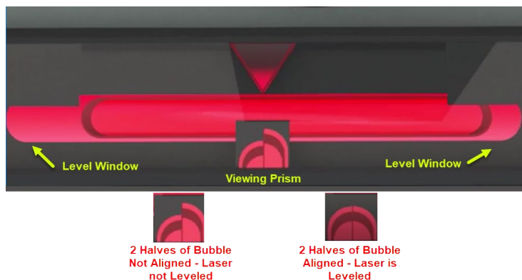
Figure 9 –L-740SP Split-Prism Level Vial Assembly for L-740 Series Lasers
