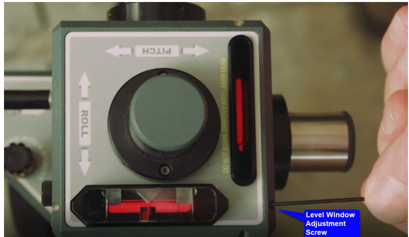
Figure 13 – L-733 (top view) showing location of Precision Level Vials and corresponding adjustment screws. Also see our YouTube video: How to Calibrate Level Vials .
