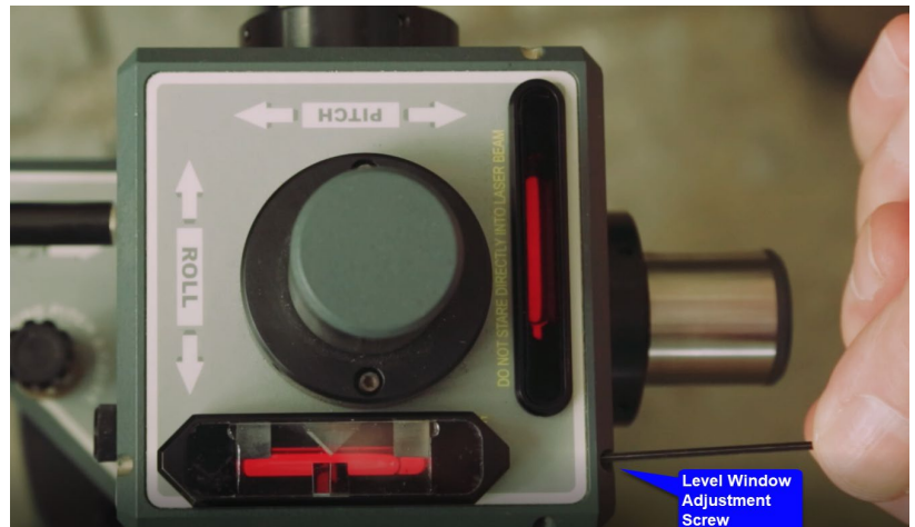
Figure 12 – L-733 (top view) showing location of Precision Level Vials and corresponding adjustment screws. Also see our YouTube video: How to Calibrate Level Vials .
