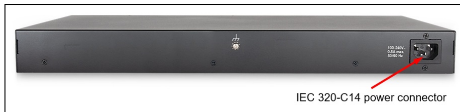
Figure 3. Rear panel of the CE0128TB switch
