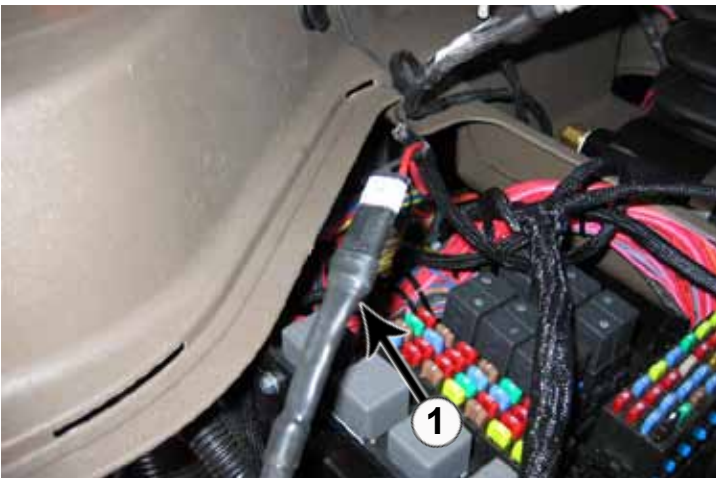
28. Connect the dozer angle extension cord (PN: 69-11663) to the wire harness (1). Run the cord through the hole in the floor of the fuse compartment.
