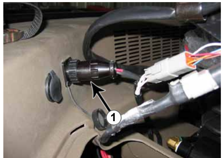
32. Plug the power cord from the wire harness into the port located behind and to the right of the operator's seat in the tractor cab (1).
