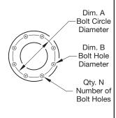
FIGURE 3 GATE VALVE FLANGE NOMINAL DIMENSIONS
