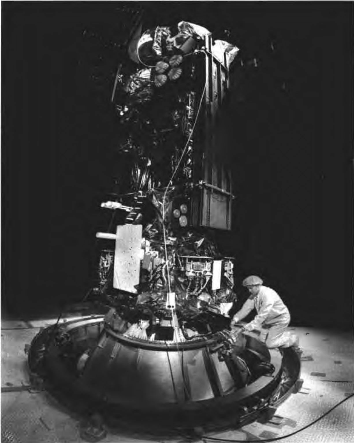
Illustration 6-2: DMSP Satellite F-16 mated to Titan II Launch Vehicle 12 January 2001 (photograph courtesy Lockheed Martin)
