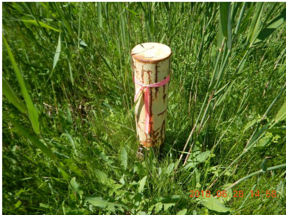
Photo 2 – Well MW1 – Casing Locked and Welded
