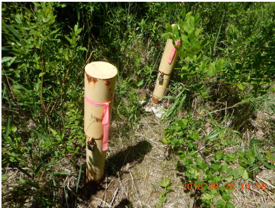
Photo 24 - Wells 99-3S and 99-3D – Casings Locked and Welded
