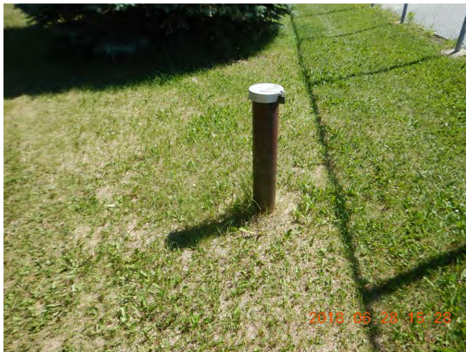
Photo 21 – Well 99-B2 – Casing Locked
