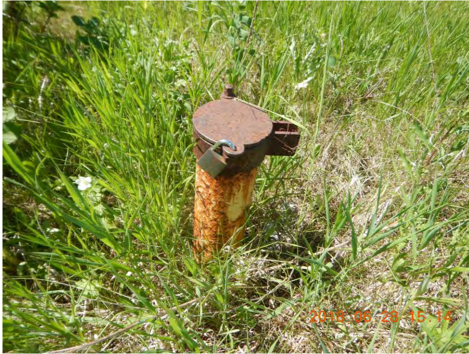
Photo 7 – Well MW7 – Casing Locked and Welded
