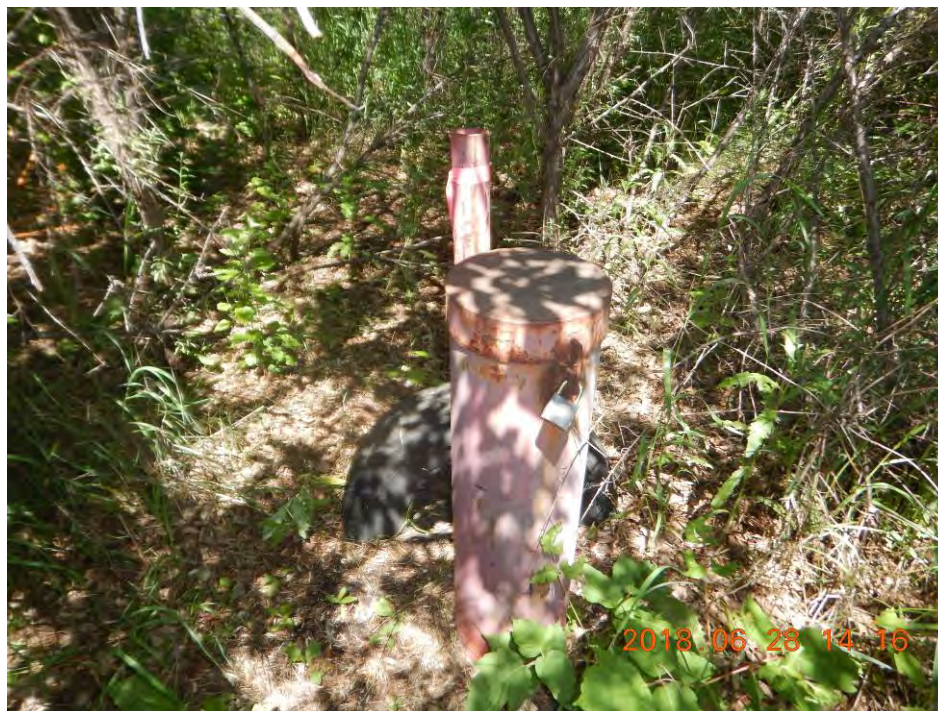
Photo 11 - Well MW11 – Casing Locked
