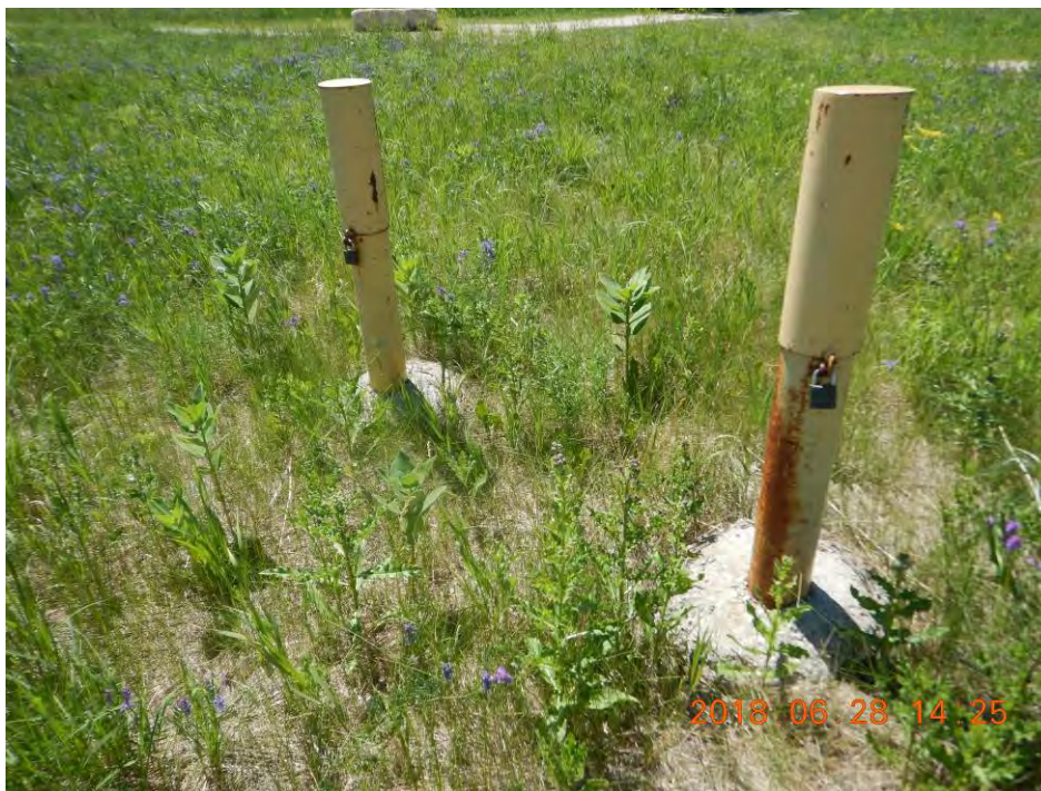
Photo 23 - Wells 99-2S and 99-2D – Casings Locked and Welded
