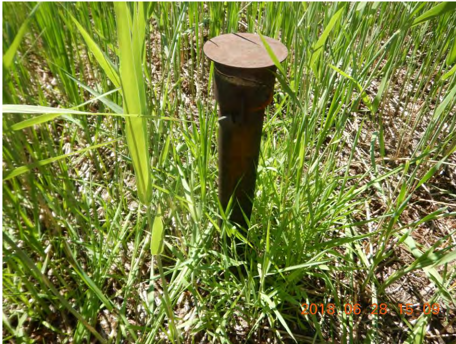
Photo 8 – Well MW8 – Casing Locked and Welded
