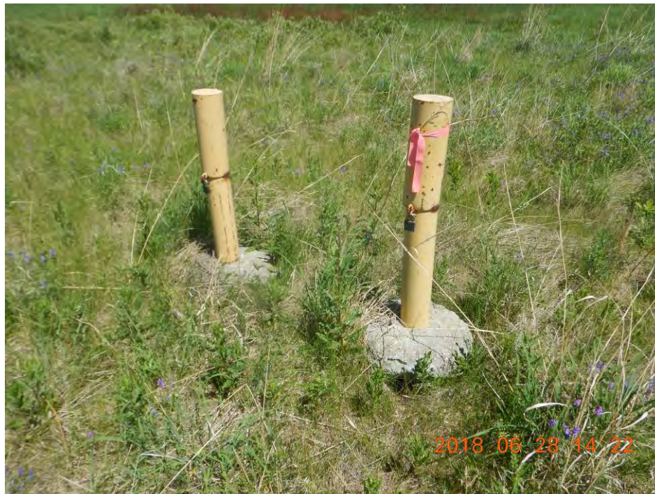
Photo 22 - Wells 99-1S and 99-1D – Casings Locked and Welded
