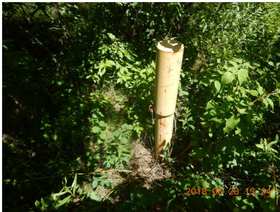
Photo 27 – Well 99-Cell-3 – Casing Locked
