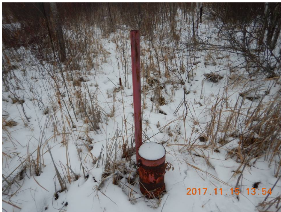
Photo 12 - Well MW12 – Casing Locked
