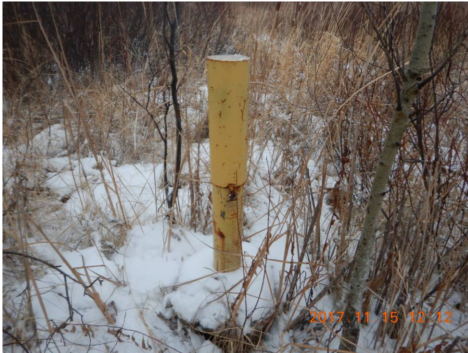
Photo 28 – Well 99-Cell-4 – Casing Locked
