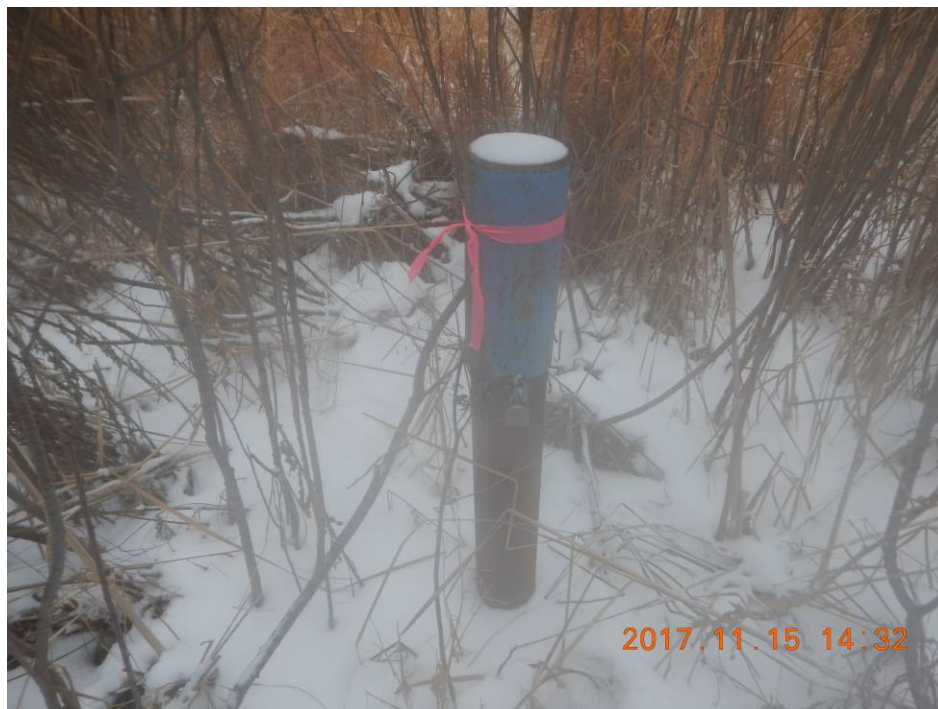
Photo 19 - Well 2002-B5 – Casing Locked and Welded
