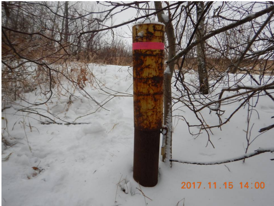
Photo 4 – Well MW3 – Casing Locked
