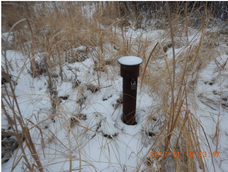
Photo 6 – Well MW6 – Casing Locked
