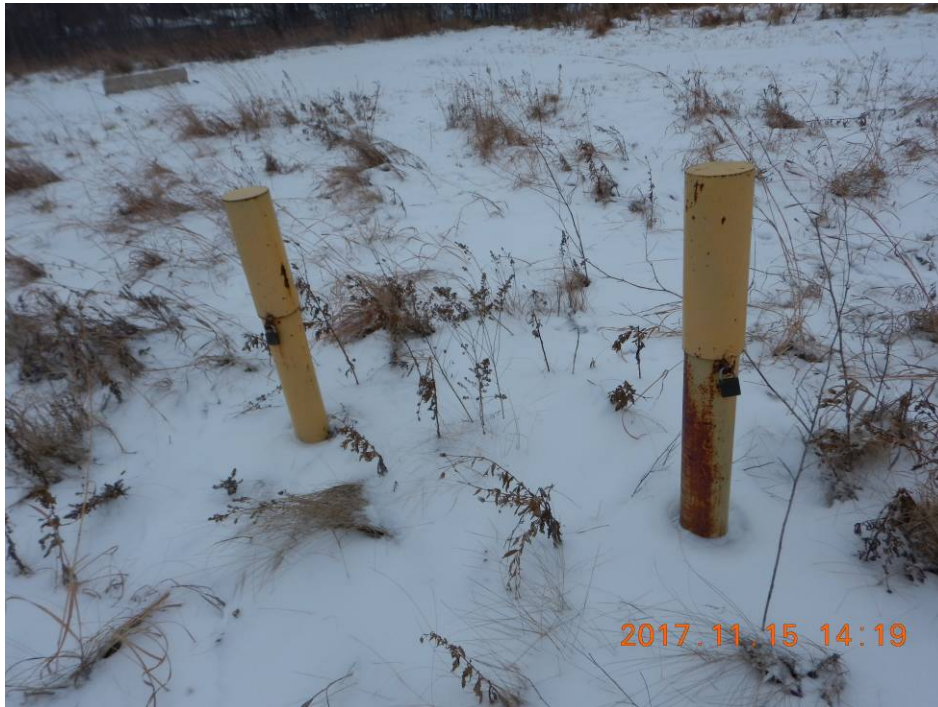
Photo 23 - Wells 99-2S and 99-2D – Casings Locked and Welded
