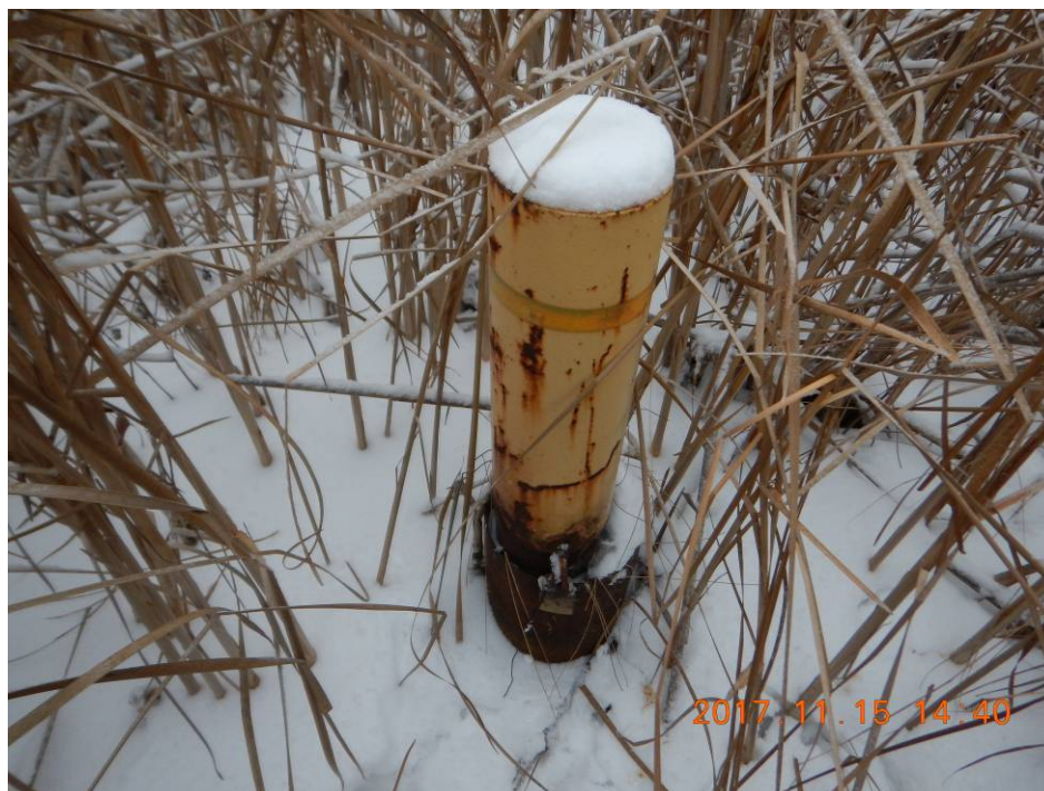
Photo 18 - Well 2000-B4 – Casing Locked and Welded
