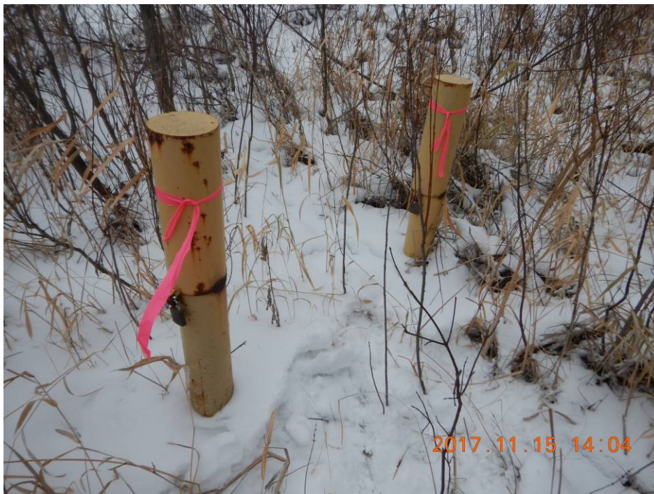
Photo 24 - Wells 99-3S and 99-3D – Casings Locked and Welded
