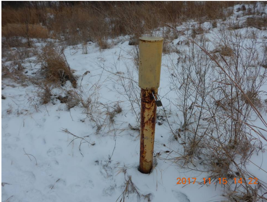
Photo 3 – Well MW2 – Casing Locked and Welded
