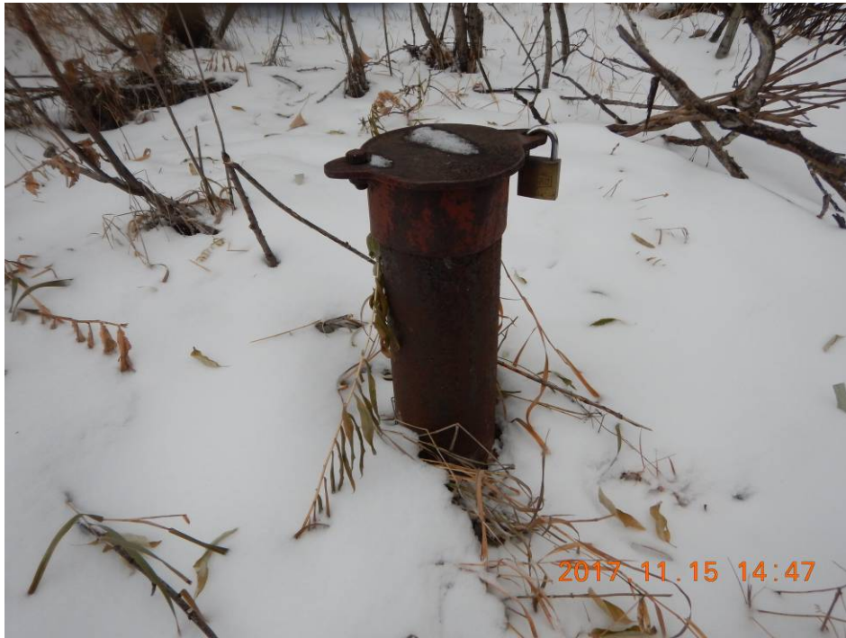
Photo 5 – Well MW4 – Casing Locked
