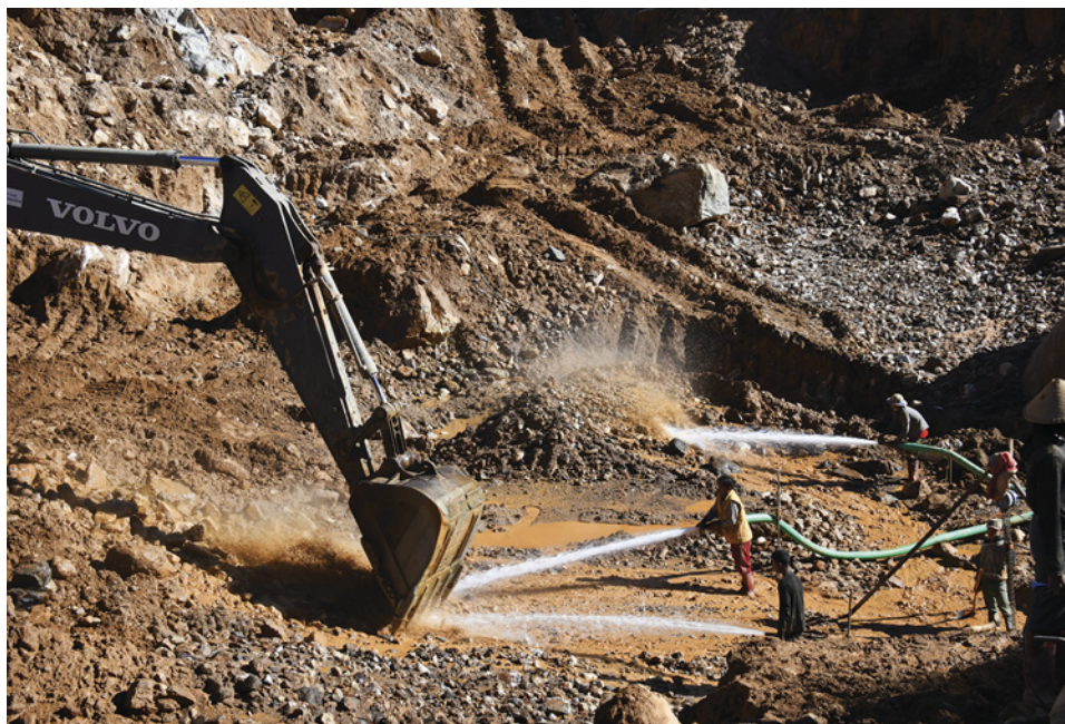
Figure 8. This modern hmyaw-dwin mine combines high-pressure water jets with an excavator. The water breaks up muddy areas, and the excavator removes large, worthless boulders and exposes fresh ground. The muddy water carries the smaller gravel and gemstones down to a gravel pump. This slurry is pumped to a washing plant, where the gems are separated from other materials. Photo by Wim Verriest.
