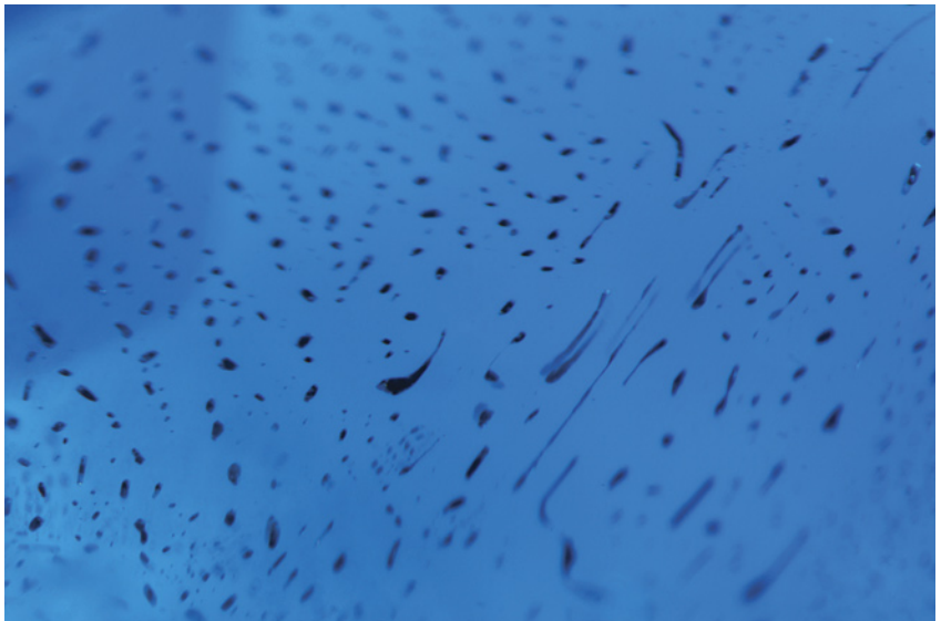
Figure 20. This flux fingerprint in the lab-grown sapphire is similar to the fingerprints found in natural sapphire. Field of view 1.76 mm.
