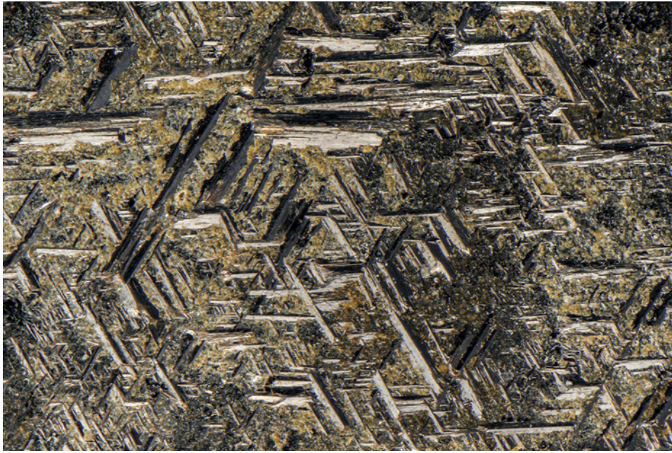
Figure 18. The sagenitic epitaxial structure of the acicular rutile crystals on the surface of this hematite gives the substrate an otherworldly appearance. Photomicrograph by Nathan Renfro; field of view 11.28 mm.
