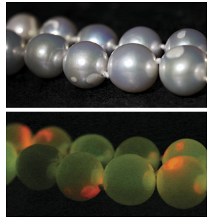
Figure 14. X-ray fluorescence analysis of the strand showed a yellowish green reaction along with a reddish orange reaction on the irregular white patches.
