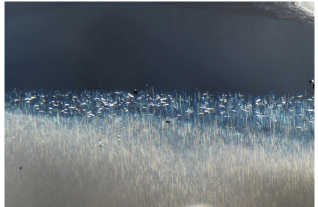
Figure 2. A myriad of inclusions at the boundary between the dense, silky core and the unincluded rim. Photomicrograph by Jonathan Moyal; field of view 1.76 mm.
