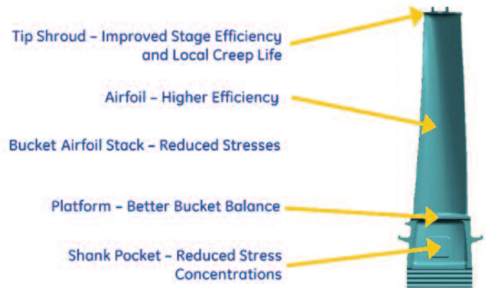
Figure 57. New stage 3 bucket design.
