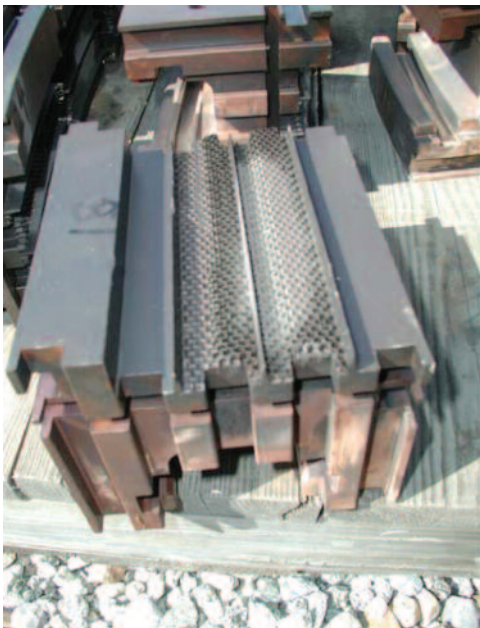
Figure 65. Shroud block with honeycomb sealing.
