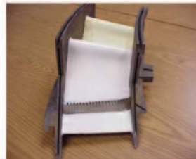
Figure 50. Design changes and reduced airflow in non-pressurized stage 2 nozzle.
