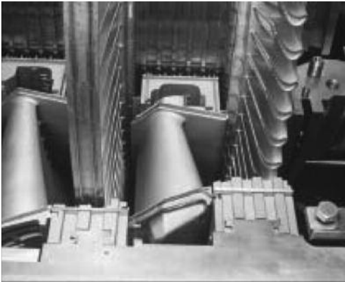
Figure 64. Stage 2 shroud blocks with honeycomb and stage 2 buckets with cutter teeth.
