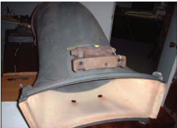
Figure 20. Nimonic 263™ transition piece for Frame 9B showing downstream aft end coated inside only with TBC.
