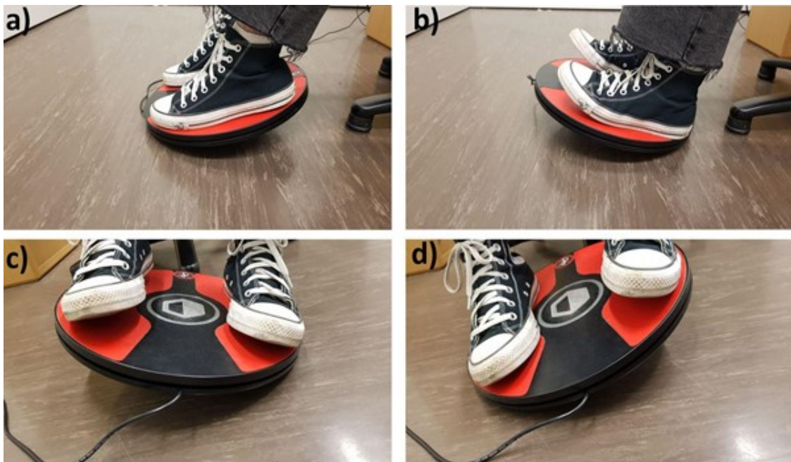
Figure 3.6 Top panel: the participant is tilting the foot-operated controller with their feet to a) move forward and b) backward through the virtual city, respectively. Bottom panel: the participant is tilting the foot controller with their feet to c) the left and d) to the right to turn their heading direction in the urban virtual city towards the left and right, respectively. The figure is adapted from Cheng et al. (2023).
