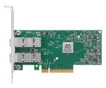
Mellanox MCX4121A-XCAT ConnectX-4 Lx EN network interface card, 10GbE dual-port SFP28, PCIe3.0 x8, tall bracket MCX4121A-XCAT
