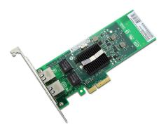
Intel Gigabit ET Dual Port Server Adapter, 82576, Dual Port, RJ45 Copper
