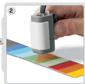
2 Hold the Light Sensor close to the different colors in your surrounding and see the different readings. You can use the color chart on page 66 of this guide or page 69 of the NXT Building Guide.
