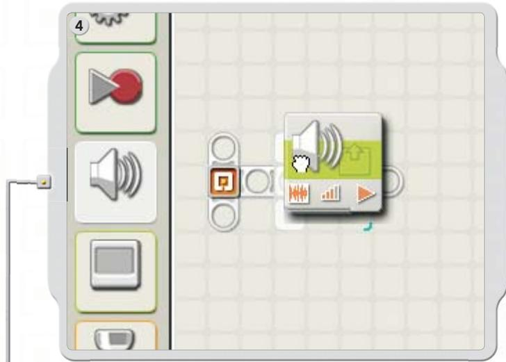
Drag a Sound block and drop it to the right of the Starting point in the work area.
