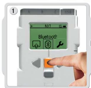
Make sure that the NXT is turned on. Also make sure that Bluetooth is set to On and that the NXT is set to Visible. (Read how in the Bluetooth Submenu on page 40). Also make sure that Bluetooth is installed and enabled on your computer.
