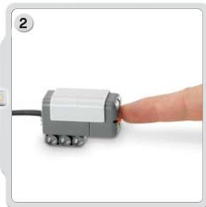
2 Make sure the Touch Sensor is in port 1. Press the Touch Sensor button.
