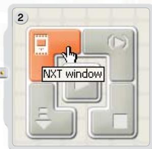
Find the Controller at the lower right work area in the software. Click on the NXT window button (the one on the upper left) and the NXT window opens.
