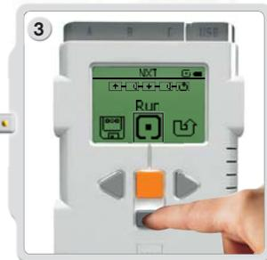
3 The program Loops continuously so press the Dark Grey button to stop the program.
