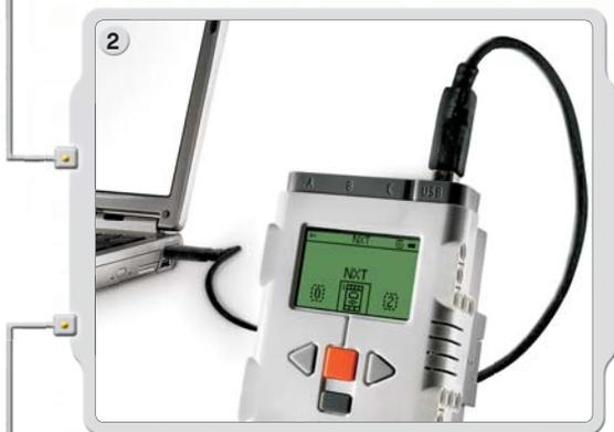
Connect the PC and the NXT with the USB cable.
