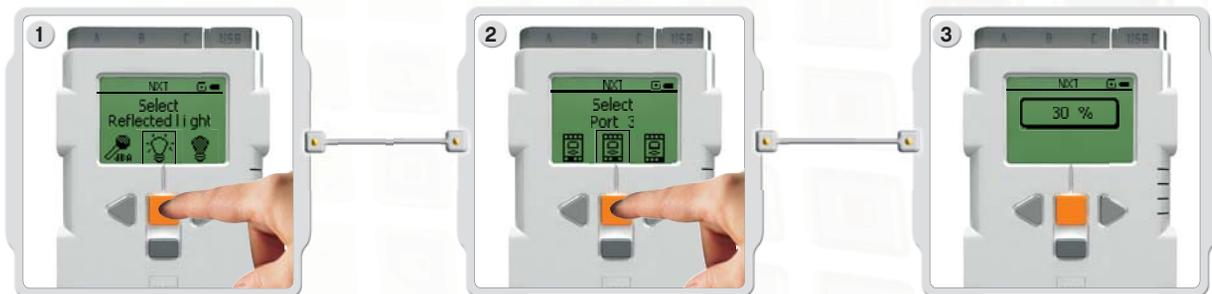
1 Select the icon of the Sensor or Motor that you want to test. You can only get readings from one sensor or motor at a time.
