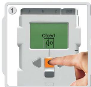
Select the Ultrasonic Sensor icon. Select the port in which you have placed the sensor.
