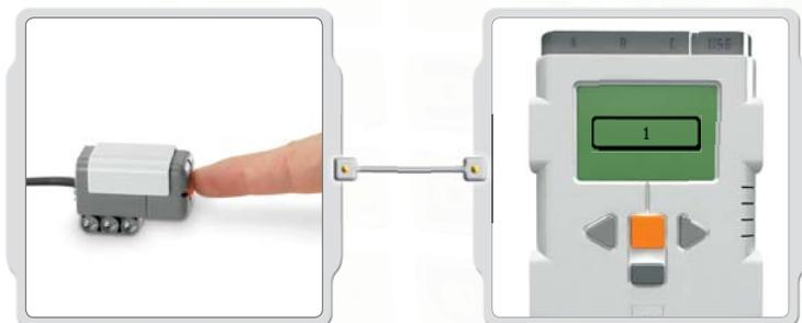
Press and hold the Touch Sensor button while watching the NXT display. You should see a one (1) on the display.
