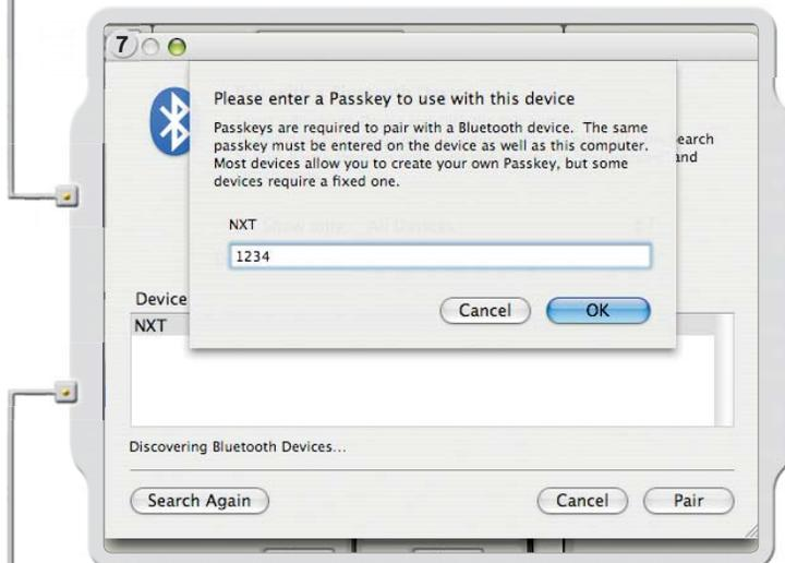
When you connect to a device for the first time, a Passkey window pops up. Enter the passkey to use with this device (the default passkey is 1234) and click OK.
