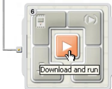
Locate the Controller in the lower right corner of the work area. Click Download and run (the center button) and listen to what happens.
