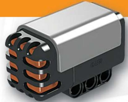
The Sound Sensor detects the decibel level: the softness or loudness of a sound. The Sound Sensor detects both dB and dBA.
