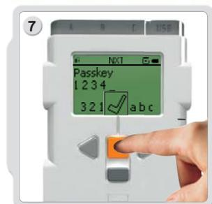
7 If you connect to a device for the first time, your NXT asks for a Passkey. Just press Enter to use the default passkey 1234 or make up your own code. The other Bluetooth device must know your passkey in order to confirm the connection. This means the two NXT bricks need to enter the same passkey in order to connect.
