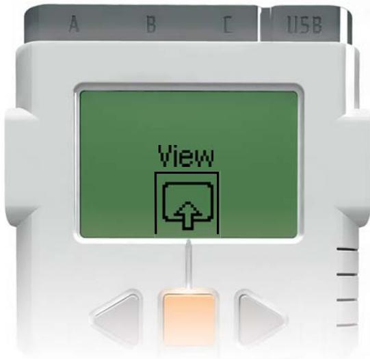
In the View submenu, you can do a quick test of your Sensors and Motors and see the current data for each.
