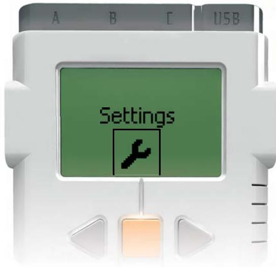
In the Settings submenu, you can adjust the different settings of the NXT, such as Loudspeaker volume or Sleep mode. In this submenu, you can also delete the programs that you have stored in the NXT memory.
