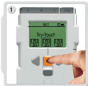
1 Press the Orange button to select Try-Touch. Press the Orange button again to Run the Try-Touch program.
