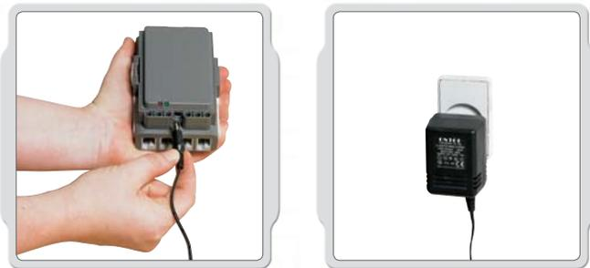
To recharge the battery, attach one end of the power adapter cord (sold separately) into the charge plug just below the NXT input ports. Attach the other end of the power adapter cord into the wall socket. The battery may also be charged when not inserted into the NXT.
