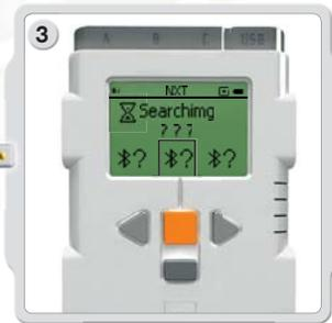
3 Depending on how many are detected in the area, the Bluetooth devices will appear in a list on the NXT display after a few seconds.
