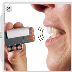
2 Make sounds into the microphone (Sound Sensor) and see the readings on the NXT. Try also to read the sounds around you: How loud are the nearest voices?
