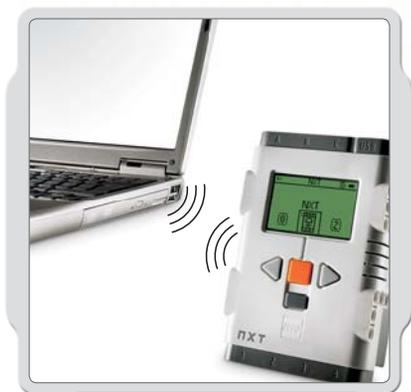
Bluetooth is a communication technology that makes it possible to send and receive data without using wires. Using the Bluetooth features, you can set up a wireless connection between your NXT and other Bluetooth devices, such as other NXT units, mobile phones, and computers.
