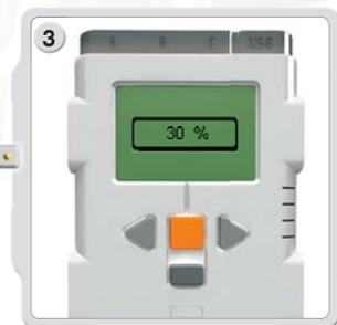
Test the Light Sensor's ability to read the surrounding light by measuring the light level in different parts of the room. For example, first hold the sensor against the window, then hold it under the table. Notice the difference in the readings. Higher numbers indicate more light (as a percentage of the light the sensor can read). Lower numbers indicate a lower amount of light.
