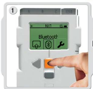
Make sure that the NXT is turned on. Also make sure that Bluetooth is set to On [On] and that the NXT is set to Visible. (Read how in the Bluetooth Submenu on page 40). Also make sure that Bluetooth is installed and enabled on your computer.
