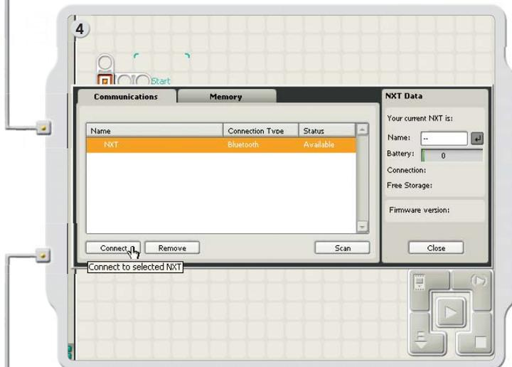
After a short interval, a list of devices appears in the window on the computer screen. Select the device to which you want to establish the connection and click the Connect button.
