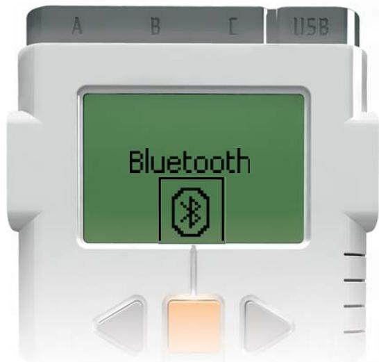
In the Bluetooth submenu, you can set a wireless connection between your NXT and other Bluetooth devices, such as other NXT units, mobile phones, and computers.
