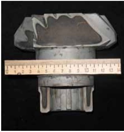
With TSH technology, parts are induction heated at low frequency and rapidly quenched, resulting in a contour induction hardening pattern (courtesy ESR Engineering Corp., North American distributor of TSH steels).
