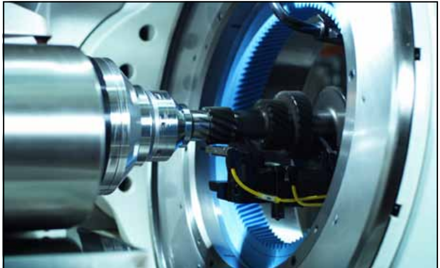
TSH technology allows difficult components, such as spiral bevel gears and pinions, to be heat treated via induction. Most of these gears are currently carburized (courtesy ESR Engineering Corp., North American distributor of TSH steels).
