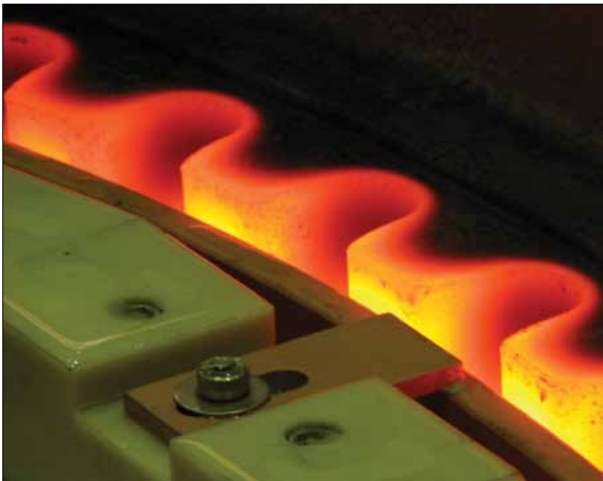
Induction Heating a large Caterpillar gear for hardening (courtesy of Caterpillar, Inc. and Ajax Tocco Magnethermic Corp).
