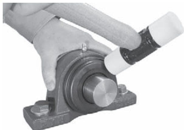
Fig. 14.13 Installing steel plate covers
