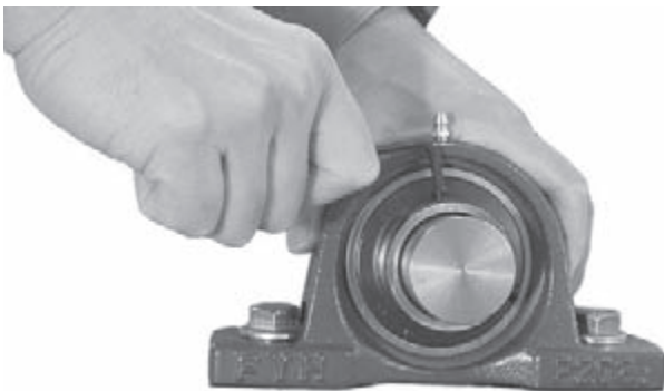
Fig. 14.5 Tightening of set screws
