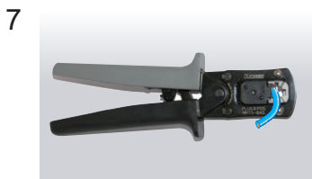
Using special crimping tool MPT5-8AS (PANDUIT CORP.), crimp the modular plug. Finally check the plug visually.
