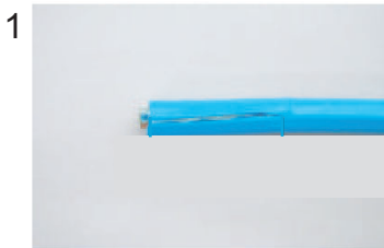
Expose inner vinyl sheath.
