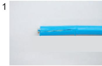
Expose inner vinyl sheath.
