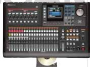
combo 1/4"-XLR jacks for line/mic in (with 48V phantom power global per 4-channels at a time), selectable guitar/hi-Z in, (2) RCA outs, (2) 1/4" balanced monitor outs, (2) 1/4" unbalanced effects sends, 1/4" headphone out, MIDI I/O for MMC, control and MTC and remote input (requires RC-3F).
