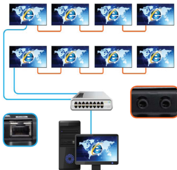
Figure 11. UDC and UEC Series displays enable RJ45 and RS-232C connectivity simultaneously.
