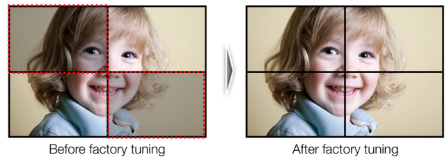
Figure 3. The side-by-side comparison demonstrates how factory tuning increases color uniformity across the video wall.
