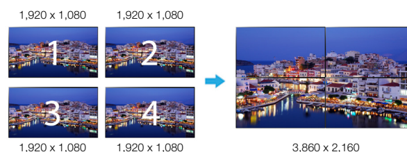
Figure 6. UDC and UEC Series displays offer UHD resolution of 3,860 x 2,160 for a 2 x 2 wall.
