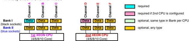
Independent Channel Mode allows all channels to be populated in any order Can run with differently rated DIMMs and use the settings of the slowest DIMM installed in the system
