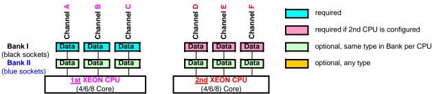
Performance Channel Mode requires identical modules on all channels of each Bank per CPU. If this mode is used, a multiple of 3 identical modules has to be ordered.
