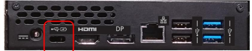
**Type-C Docking Port: one single cable to operate ESPRIMO G558**
