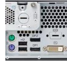
Up to 3 **digital display** onboard for ergonomic working, VGA connector as option
