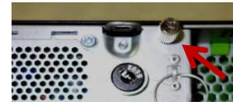
**Tool less** opening with Thumb screw
