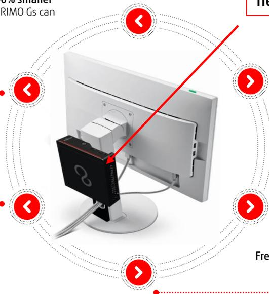
ESPRIMO G558 mounted to an 8th Generation professional display using new mounting plate
