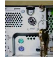
Optional **integrated cabinet lock**, hole for pad lock and Kensington as standard for security
