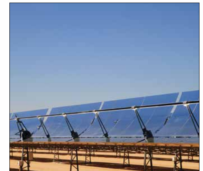
Nook worm gear screw jacks used in a solar application.
