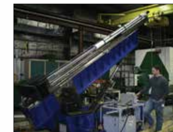
Convertible Test System 20,000 lb load - 100" CC
