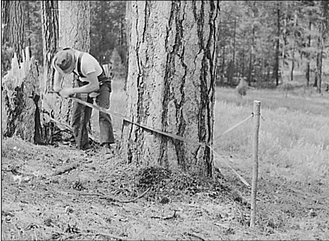
Figure 53 – Falling a large ponderosa pine by using a crosscut saw and a ‘rubber-man’ setup in Grant County, Oregon (photo by Russell Lee, July 1942). In this situation, a single faller could work a tree by driving a stout stake in the ground, and then attaching strips of rubber inner tube to the stake and one end of a saw. A faller would pull the saw, and a ‘rubber-man’ would pull it back.
