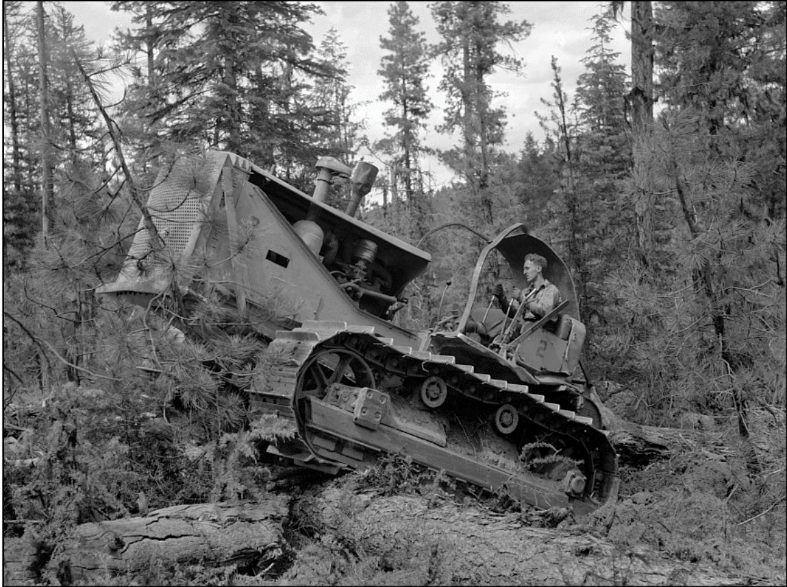
Figure 55 – Yarding ponderosa pine logs after they were felled and bucked into merchantable lengths; Grant County, Oregon (photo by Russell Lee, July 1942). During this era, crawler tractors were commonly used to haul bucked logs to a collection point where a larger tractor would then skid them to a loader (fig. 56). It was subsequently learned, however, that crawler tractors often caused unacceptable levels of soil compaction (Froehlich and McNabb 1984), depending on soil type, soil moisture, and other factors.
