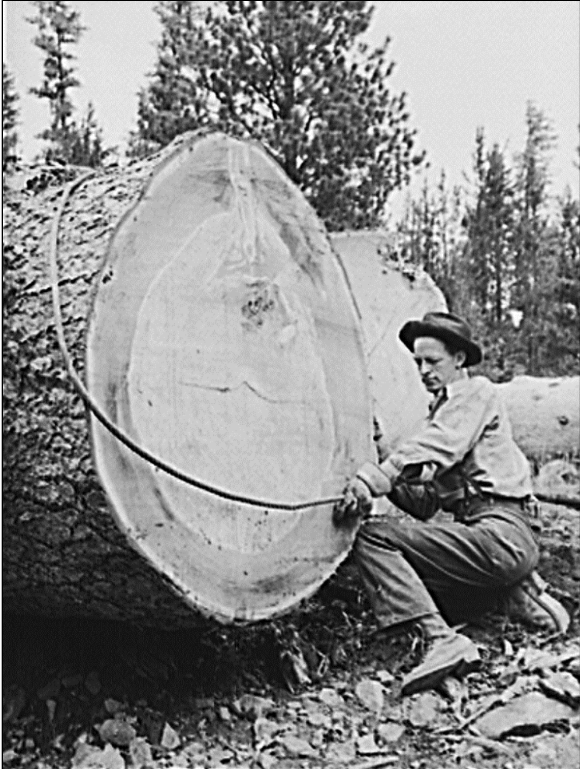
Figure 54 – Setting a choker cable on a large pine log in Grant County, Oregon (photo by Russell Lee, July 1942). This image shows very large size associated with centuries-old ponderosa pines being removed from Bear Valley Unit by Edward Hines Lumber Company.
