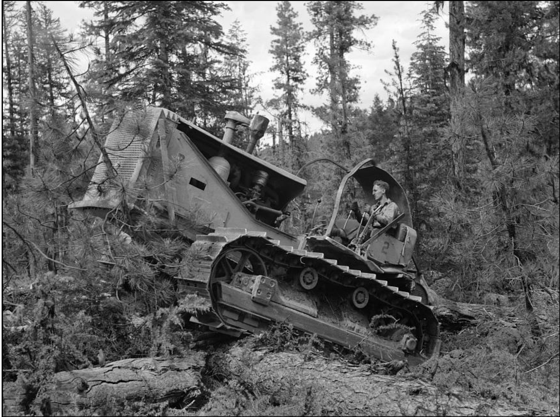
Figure 55 – Yarding ponderosa pine logs after they were felled and bucked into merchantable lengths; Grant County, Oregon (photo by Russell Lee, July 1942). During this era, crawler tractors were commonly used to haul bucked logs to a collection point where a larger tractor would then skid them to a loader (fig. 56). It was subsequently learned, however, that crawler tractors often caused unacceptable levels of soil compaction, depending on soil type, soil moisture, and other factors.
