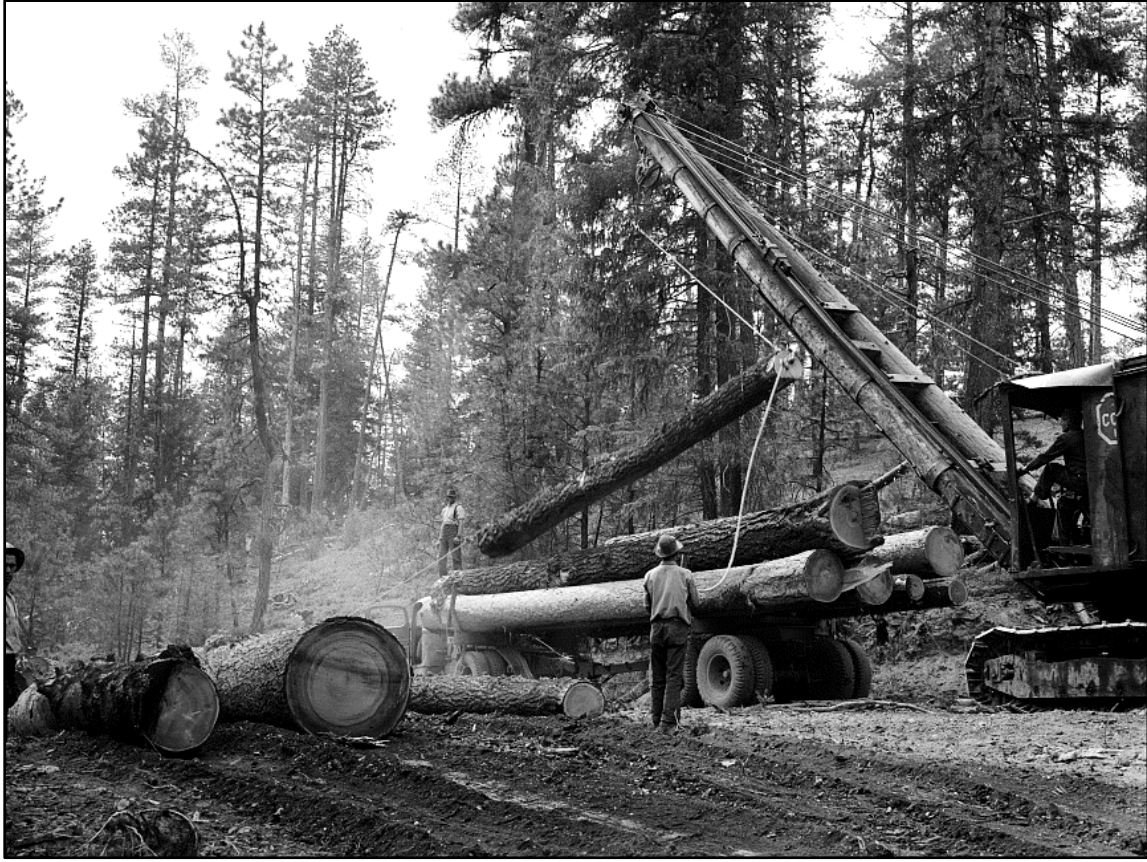
Figure 57 – Loading ponderosa pine logs on a truck for transport to a mill yard in Grant County, Oregon (photo by Russell Lee, July 1942). After a large crawler tractor delivers its load of logs to a loading area (fig. 56), a boom-type loader lifts them up and swings them over to a log trailer, where they are added to a load in preparation for transport to a mill yard in town.
