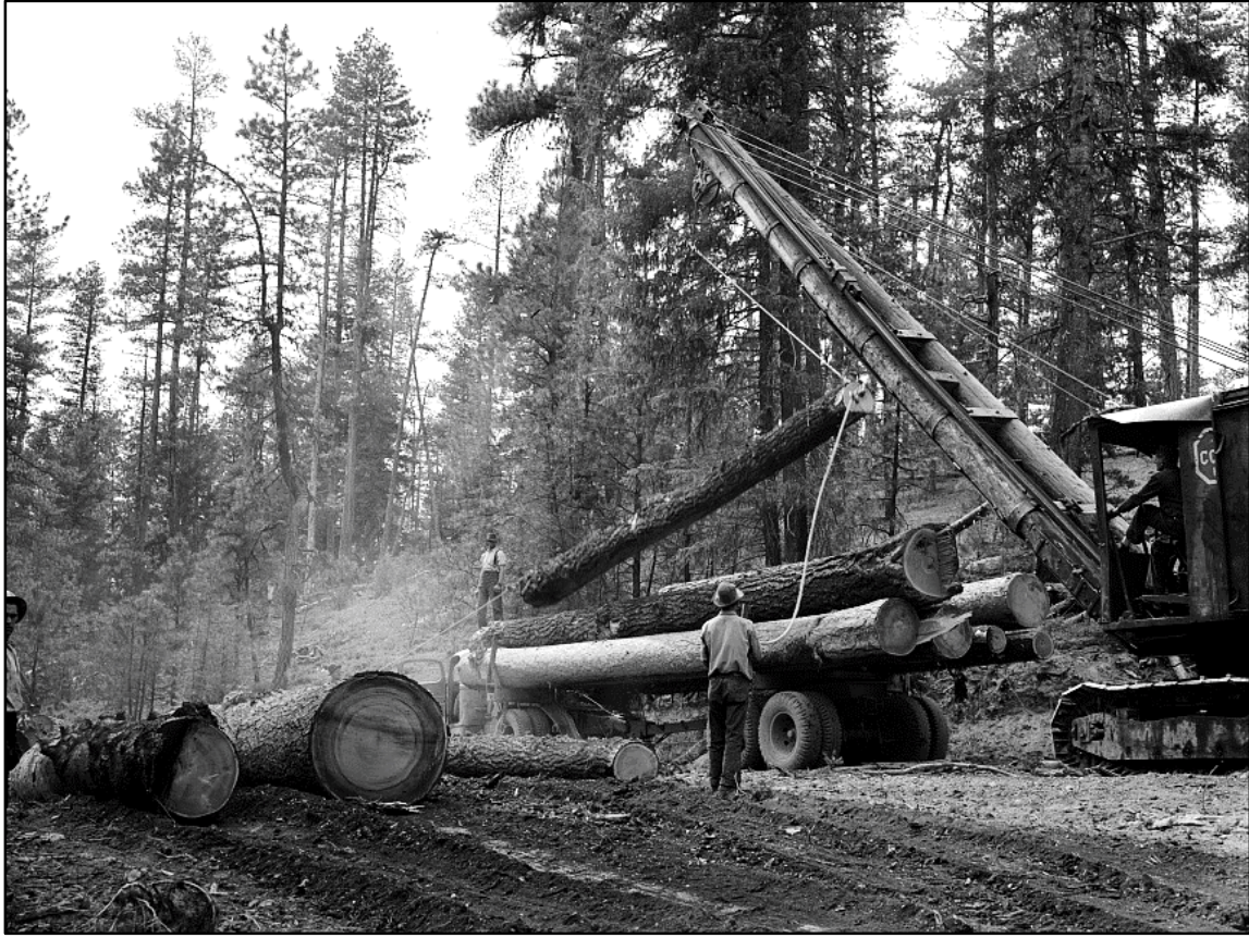
Figure 55 – Loading ponderosa pine logs on a truck for transport to a mill yard in Grant County, Oregon (photo by Russell Lee, July 1942). After a large crawler tractors delivers its load of logs to a loading area (fig. 54), a boom-type loader lifts them up, and then swings them over to a log trailer, where they can be placed on the load in preparation for transport to the mill yard in town. Once again, note the mixed-species composition of the background forest stand, and a high level of soil disturbance in the foreground scene.
