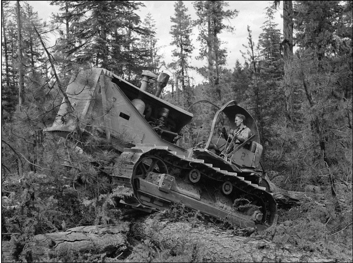
Figure 53 – Yarding ponderosa pine logs after they have been felled and bucked into merchantable lengths; Grant County, Oregon (photo by Russell Lee, July 1942). During this era, crawler tractors were commonly used to haul bucked logs to a collection point where a larger tractor would then skid them to a loader (fig. 54). It was subsequently learned, however, that crawler tractors often caused unacceptable levels of soil compaction, depending on soil type, soil moisture, and other factors. Note that the surrounding stand contains some tree species other than ponderosa pine, although sale contracts of this era typically did not require their removal, or their removal was at the discretion of the purchaser.
