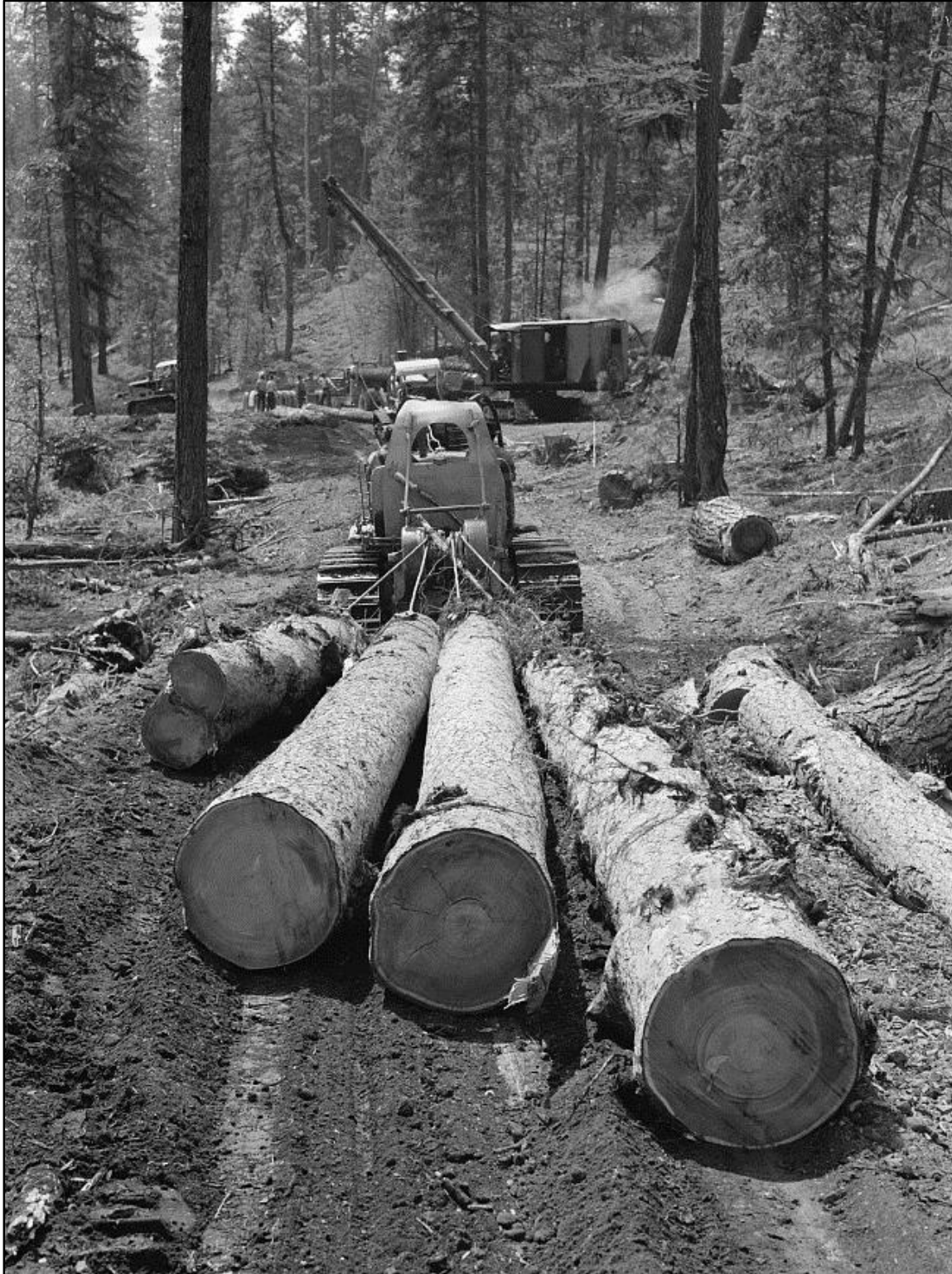
Figure 54 – Skidding logs to a loader in Grant County, Oregon (photo by Russell Lee, July 1942). As noted for figure 53, this photo depicts a surrounding stand containing tree species other than just ponderosa pine. In fact, the tractor is approaching a western larch on its right side with dwarf mistletoe infection in its lower branches. Note the high level of soil disturbance associated with these major skid trail routes.
