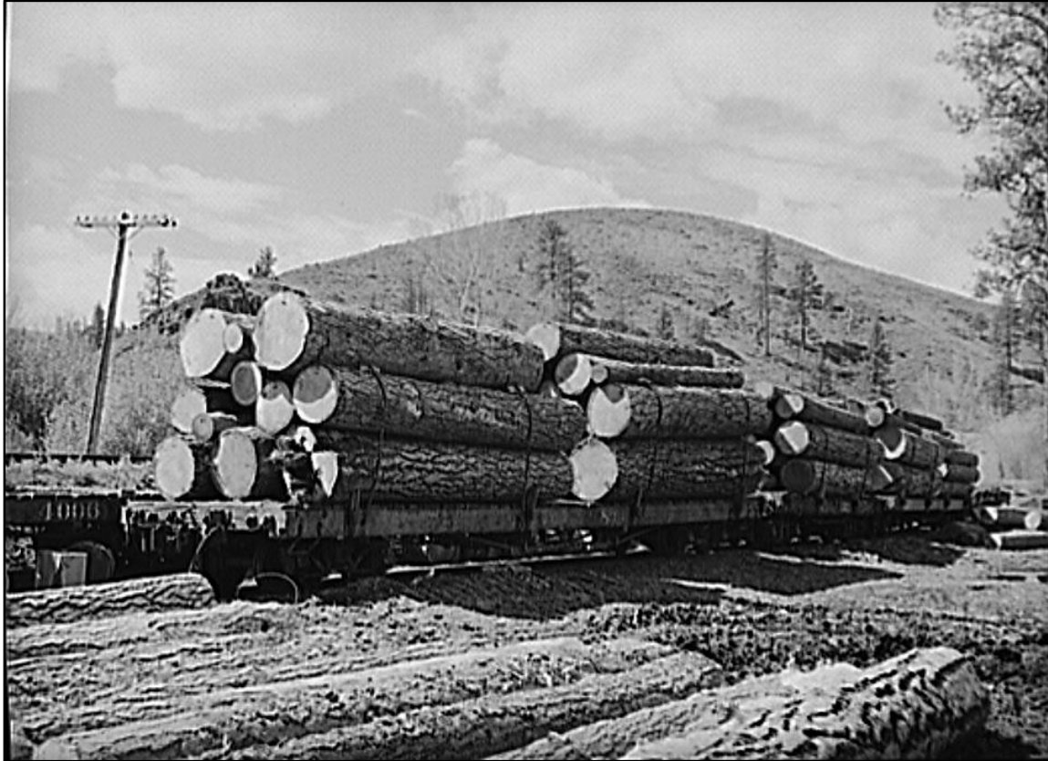
Figure 57 – Loading large ponderosa pine logs onto railroad cars in Baker County (photo by Russell Lee, 1941). As noted at the beginning of this section, railroad logging was not uncommon in the Blue Mountains, particularly in association with high-volume timber sales such as the Bear Valley Unit. Most of the logging railroads (and they were plentiful) were narrow-gauge, although the track and ties have now been removed and little evidence remains of their existence, other than an abandoned rail bed.
