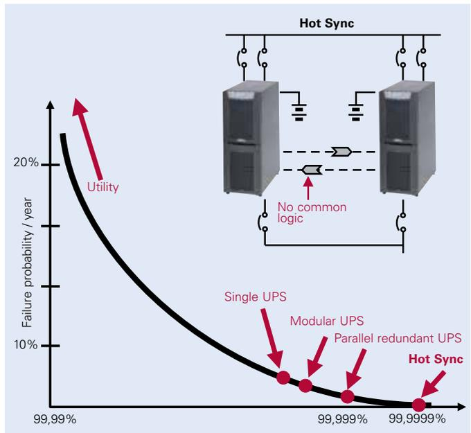
Figure 1. Power availability with various power supply configurations.
